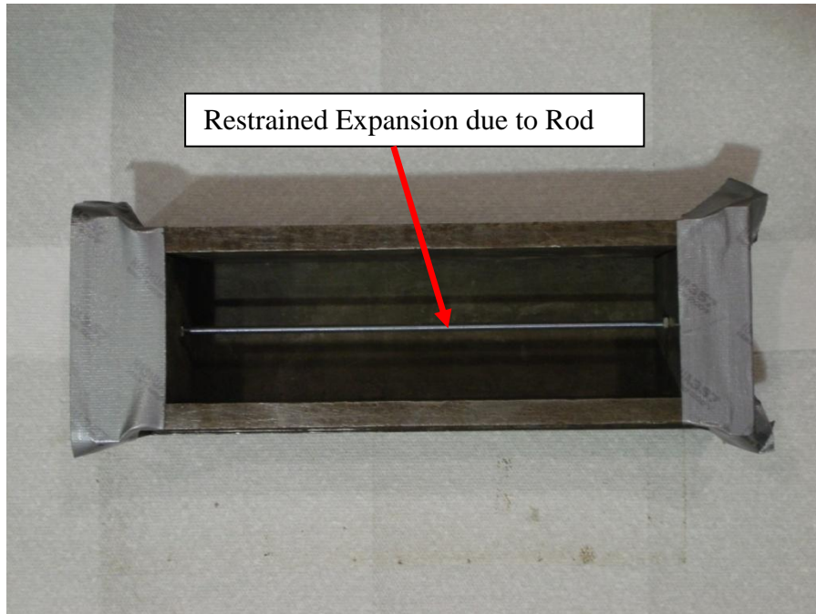
Figure D.16 Prism form was used for ASTM C 878 restrained expansion method
