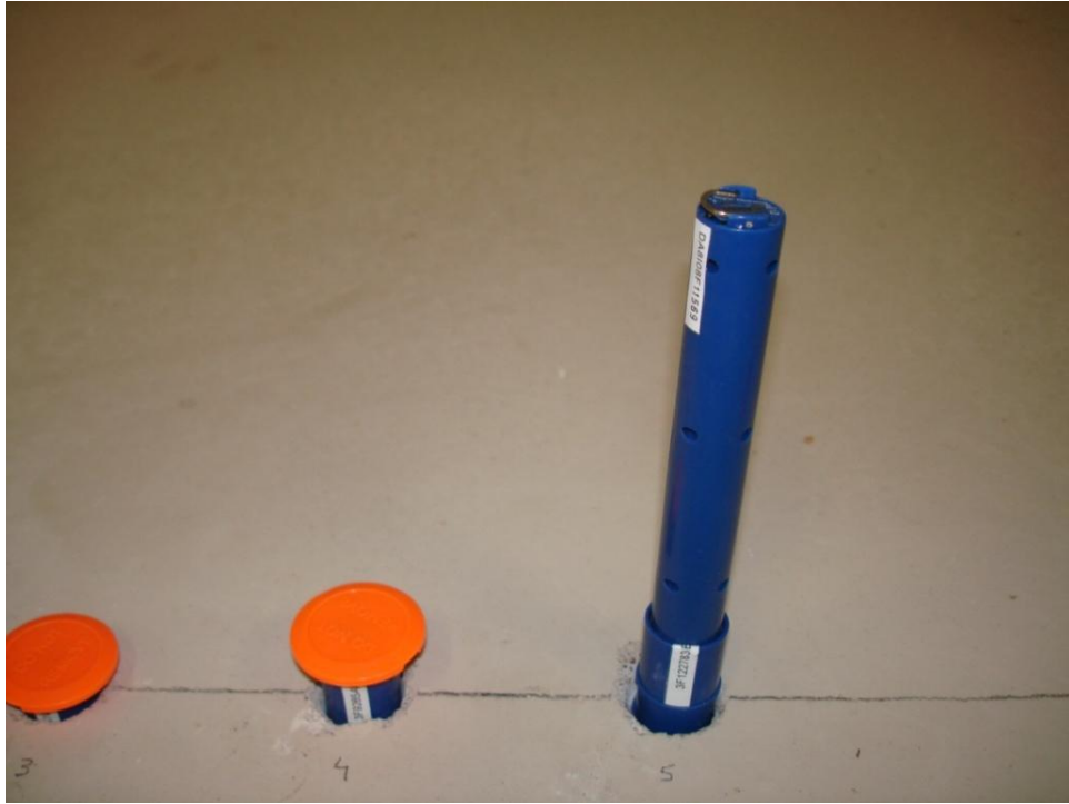
Figure 3.33 Slab internal temperature and moisture meter
