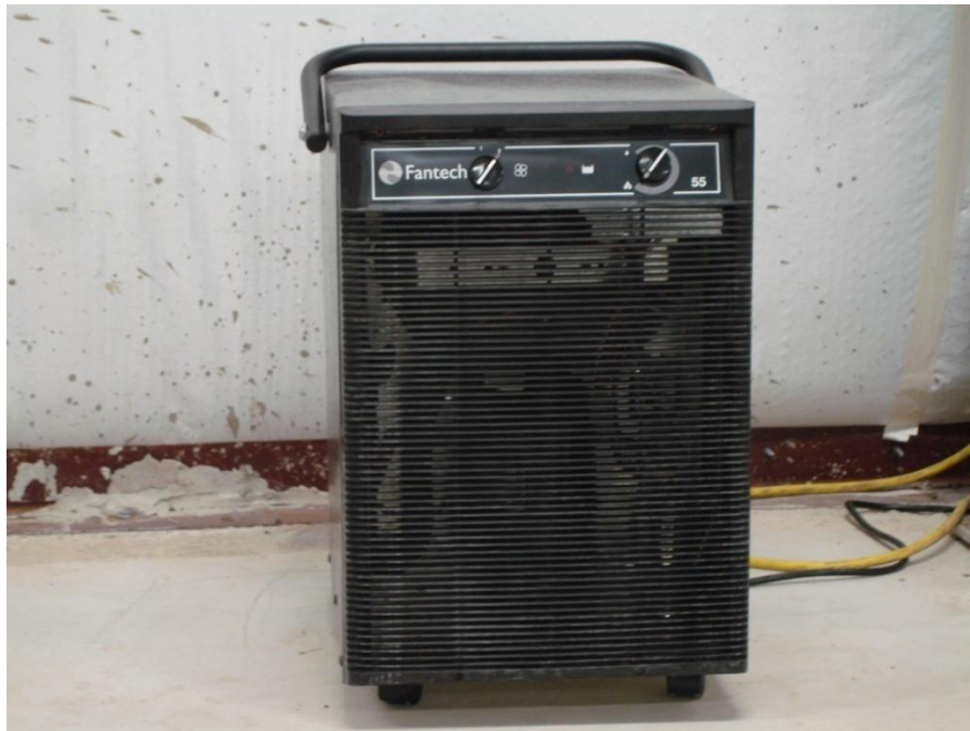
Figure 3.46 Dehumidifier used to reduce the ambient relative humidity
