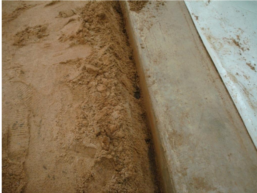
Figure D.1 Making gap into the sand at the sides of the slab specimens to place the Foam around the slab specimens
