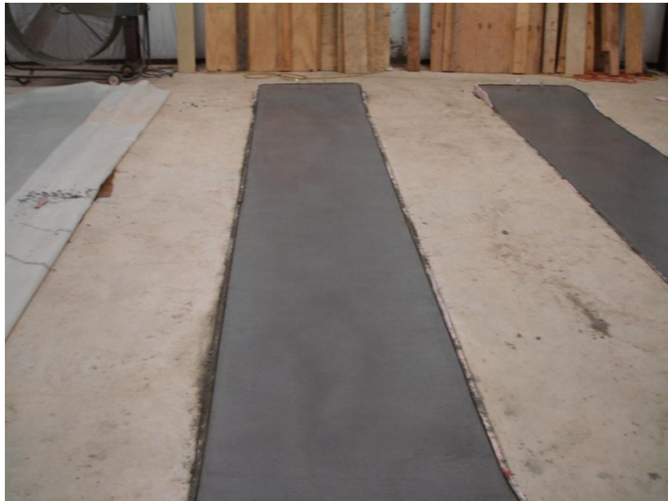
Figure 3.24 Finished concrete slab specimens
