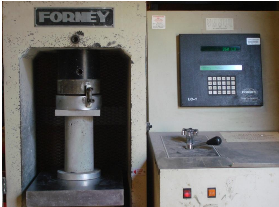
Figure 3.31 Cylinder specimens placed for testing the compressive strength of concrete
