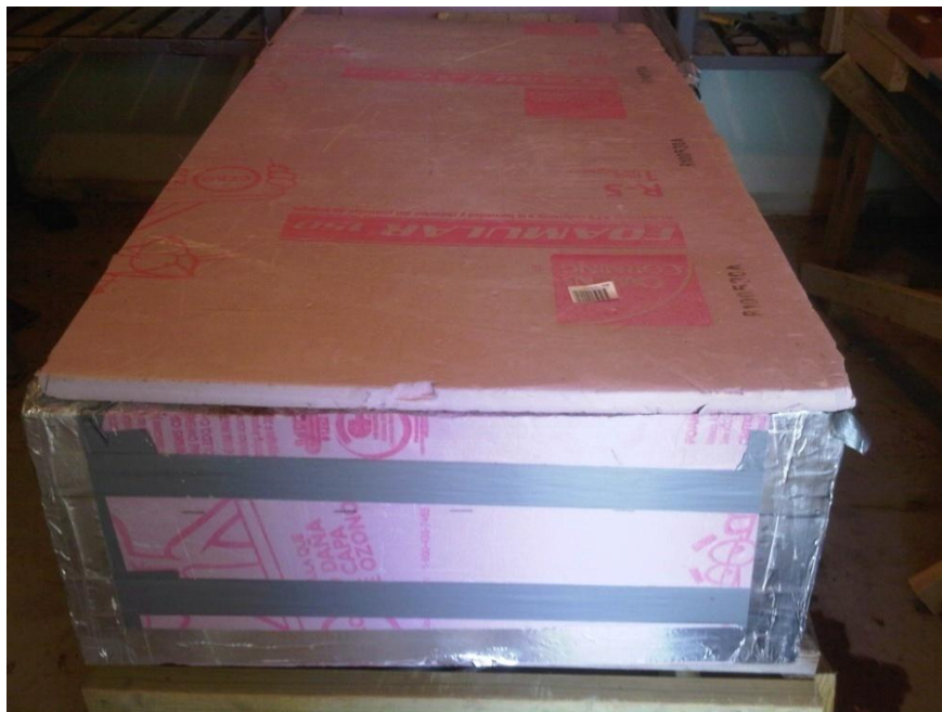
Figure D.21 Placed specimens in a closed box to keep Humidity during the curing time
