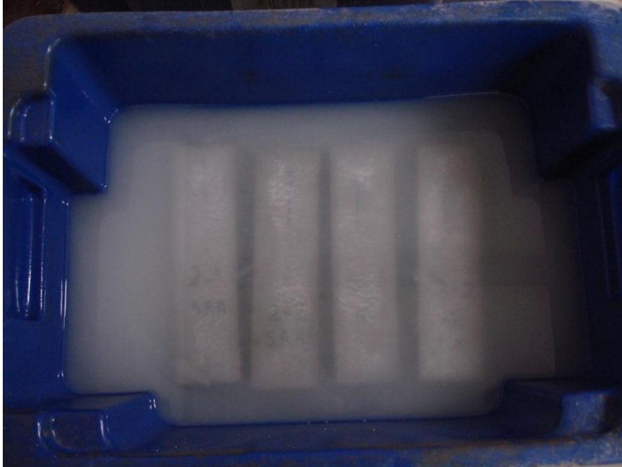
Figure D.18 Cured specimens for 7 days in water and limestone
