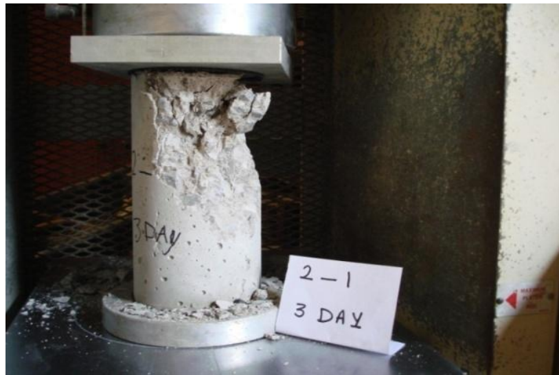
Figure 3.5 Compressive strength test (ASTM C 39)
