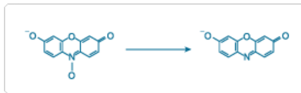
Figure 16: Chemical mechanism illustrating the reduction of the resazurin dye when in the presence of metabolic active cells [122].
