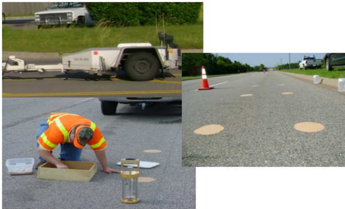
Figure 2.2 ODOT Skid Trailer, Outflow meter ASTM STP 583 and the Transit New Zealand TNZ T/3 Sand Circle Testing.
