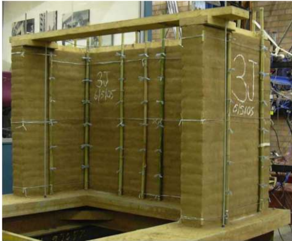
Figure 4.15. Adobe test structure with bamboo external reinforcing (Samali et al 2006)
