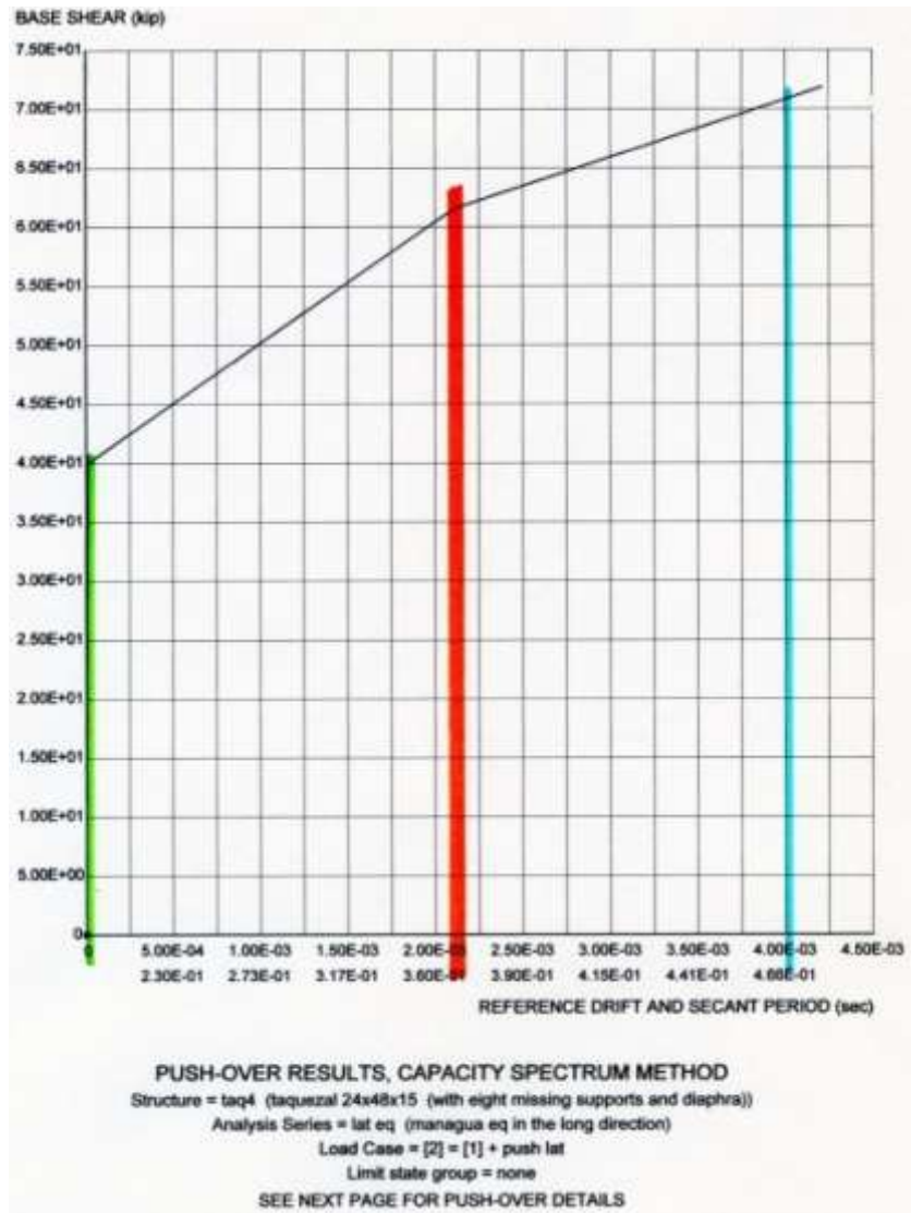
Figure 8.66. Taquezal building with weak supports – longitudinal pushover analysis
