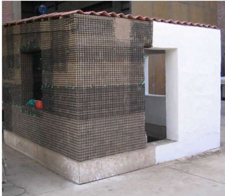
Figure 4.17. Adobe test structure with mesh reinforcement (Blondet 2006)
