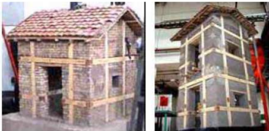
Figure 4.16. Adobe test structure with wood reinforcement (Yamin et al 2004)
