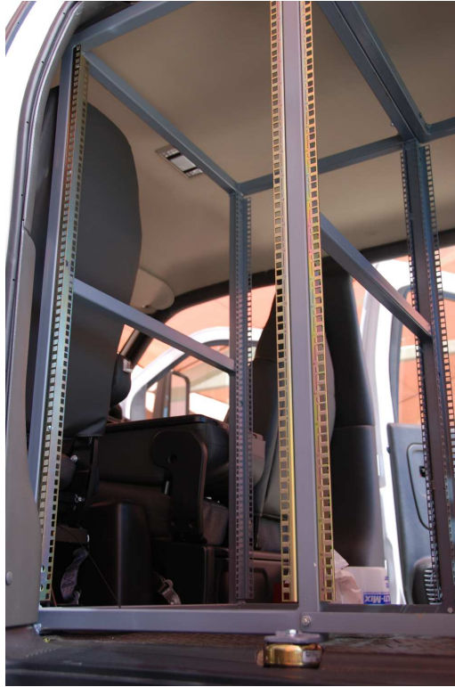
Figure 4.14: A complete computer rack within the AIR truck cab. The metal cylinder at the base of the rack is a shock absorber designed to minimize vibrations on sensitive computer equipment.
