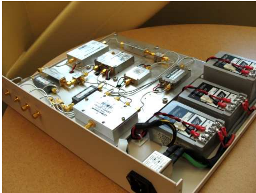
Figure 4.25: A photograph of the completed up conversion unit. DC voltage is distributed by three, on-board power supplies. The inputs, located on the front panel, are a 80-MHz clock input, 50-MHz IF input, 9550-MHz RF output, 240-MHz clock output, and an 80-MHz clock output.
