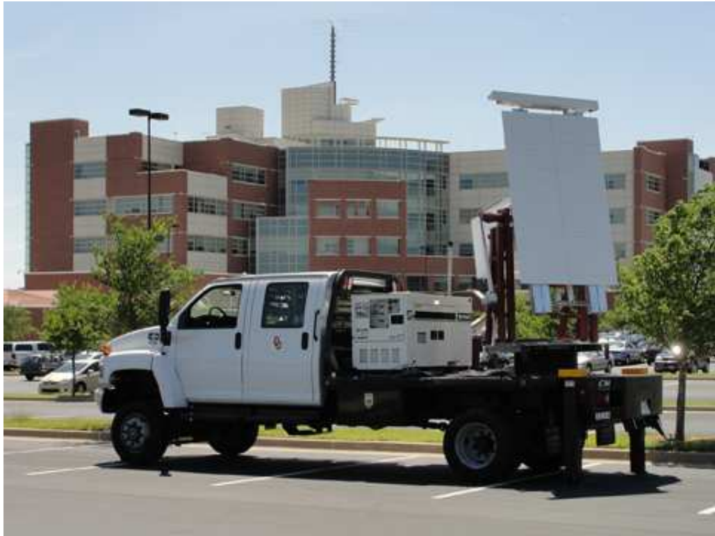
Figure 4.1: An image of the AIR mobile radar. The completed system is comprised of multiple subsystems divided into the pedestal, array, transmit, receive, and digital storage assemblies. Each subsystem will be discussed in detail and results from subsystem tests are presented.
