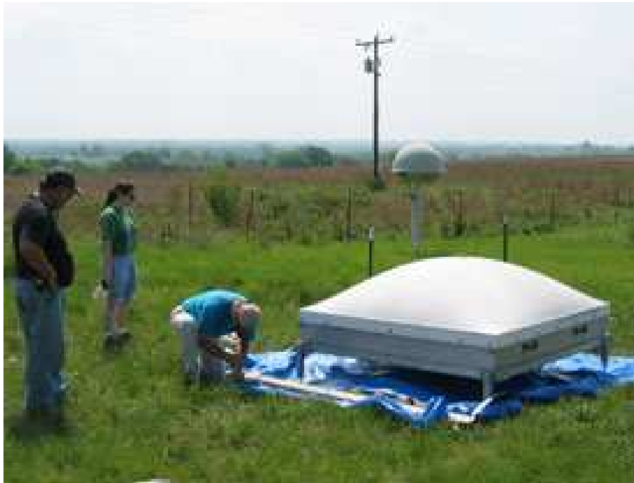
Figure 1.3: Installation of the wind profiler located at Kessler Atmospheric and Ecological Field Station ( http://kff1.ou.edu ). The wind profiler operates at 915 MHz and 500 W peak power.
