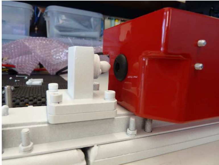
Figure 4.32: An image of a down conversion enclosure mounted on a subarray. The waveguide to SMA adapter port aligns with the input grommet on the enclosure. A diode limiter attaches to the SMA port and enters the box through the grommet.
