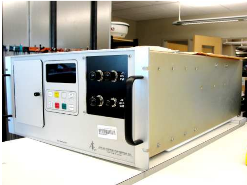
Figure 4.26: A photograph of the TWT amplifier prior to installation. The forward and reverse sample ports are located on the front of the device while the waveguide output and RF and trigger inputs are on the back. A control interface is also located on the front panel with a display indicating the amplifier status.
