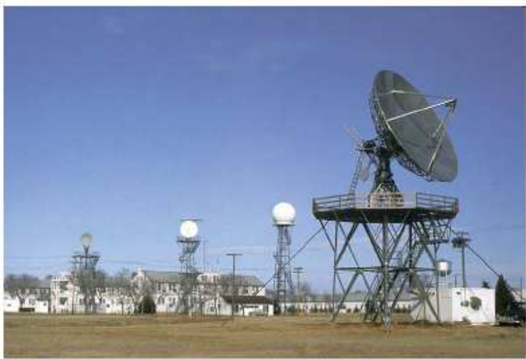
Figure 1.8: Image of the NSSL Doppler radar in Norman, Oklahoma (Brown and Lewis 2005). Also shown are the WSR-57 research radar and two aircraft tracking radars. It was through this testbed that the modern era of weather radar technology was developed and evaluated. A similar system was constructed in Cimarron, Oklahoma.
