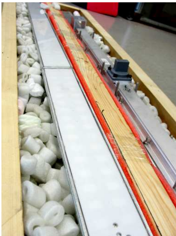
Figure 4.29: A photograph of the two prototype subarray assemblies. The subarrays themselves are comprised of an array of patch antennas combined in series. Identical 2 \times 36 element arrays are combined in the center to form the full subarray. A waveguide to SMA adapter serves as the output port.
