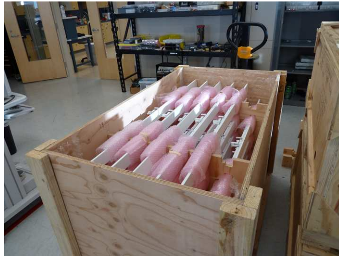
Figure 4.30: A photograph of the 36 production subarrays. The final design had an upgraded structure for added stability and a painted radome for UV and weather protection. The down conversion units attach to the back of the subarray assemblies.
