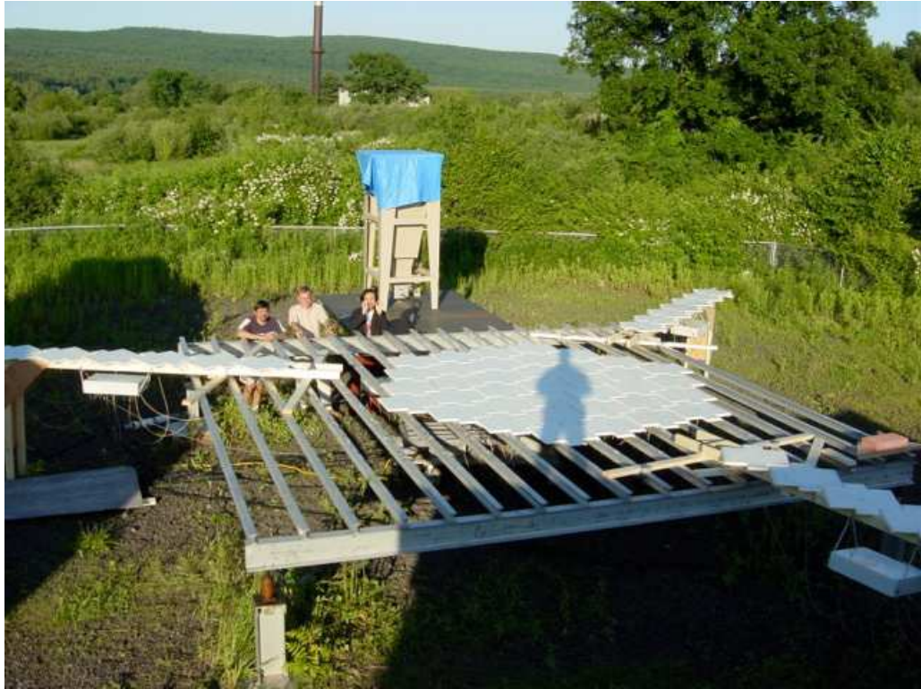
Figure 1.5: An image of the TEP radar at UMass (courtesy of Dr. Robert Palmer). Each of the panels for this 915 MHz imaging wind profiler can be rearranged to examine the effects of alternative array patterns. Further, the use of digital beamforming allows for adaptive algorithms to enhance the quality of the radar signals.
