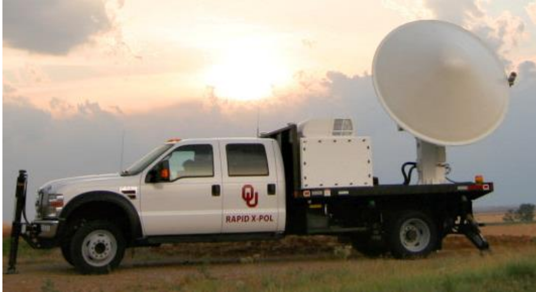
Figure 18: The rapid-scanning, X-band, polarimetric radar (RaXPOL) (Photo courtesy of J. Snyder.)
