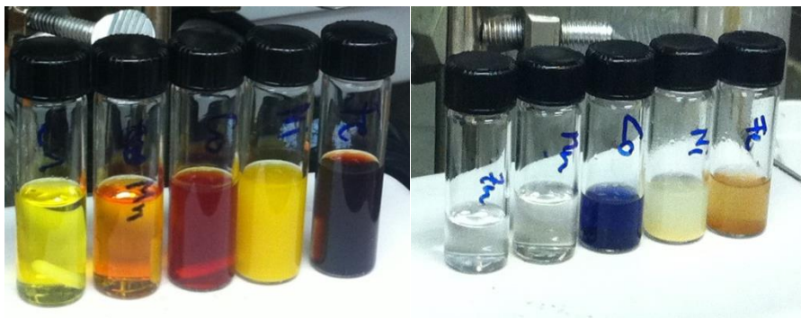
Figure 4.29. Left: colored solutions of divalent metal ions with \text{H}_2\text{L}^{5\text{-ortho}} (Zn, Mn, Co, Ni, Fe: from left to right). Right: solutions of the corresponding metal ions in methanol.
