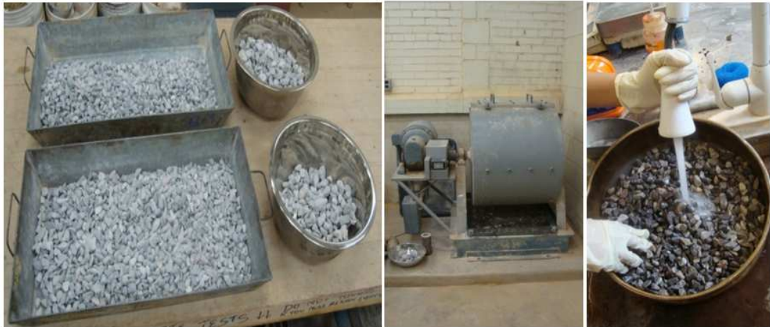
Figure 6.3. Los Angeles (LA) abrasion tests
