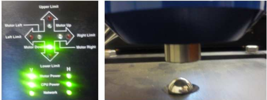
Figure 6.14. (a) Front panel of the DST machine (b) Positioning of the vertical load cell on the test cell
