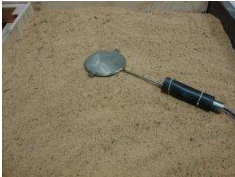
Figure 8.9. An earth pressure cell was placed on a 25 mm sand layer on top of the aggregate
