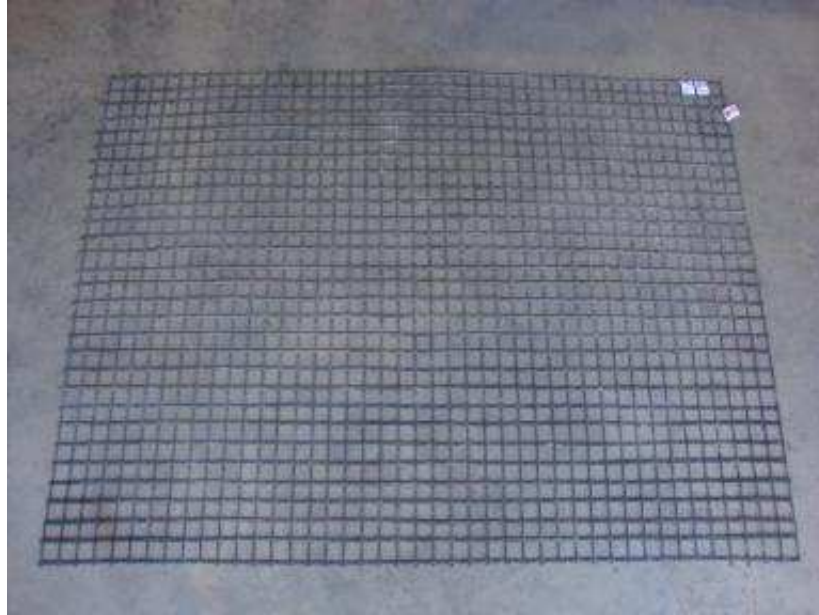
Figure 7.38. WGG1 geogrid specimen after exhumation
