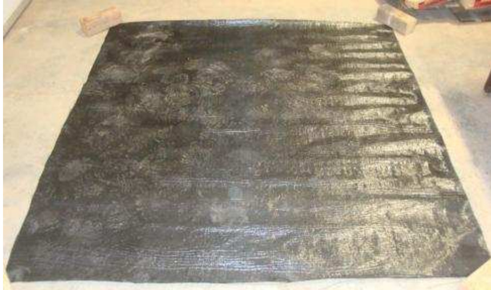
Figure 9.25. Geotextile placed below the subgrade layer in the test box
