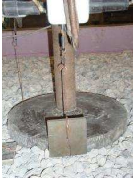
Figure 9.42. Vertical telltale plate to measure the aggregate deformation near the circular loading plate
