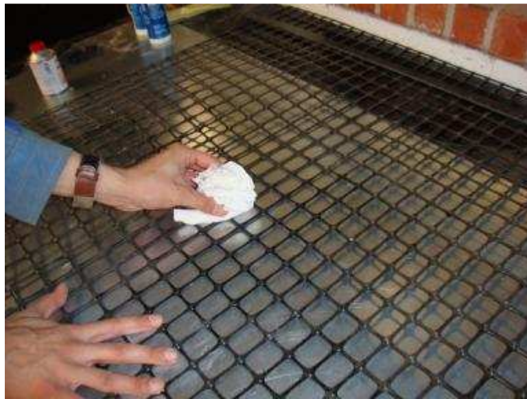
Figure 9.9. Cleaning the surface of geogrid with industrial tissue or cloth
