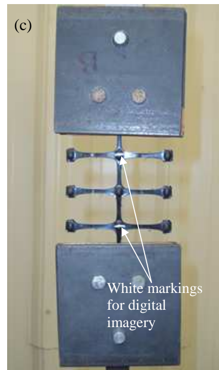
Figure 5.3. (a) Geogrid specimen secured in the clamps, (b) test setup mounted on the tension frame, (c) view from digital camera, ready to record the specimen deformation
