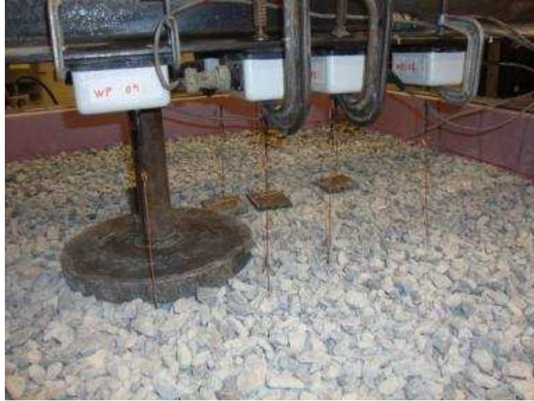
Figure 9.39. Brass wires connected to the wire potentiometers to measure the base layer deformation
