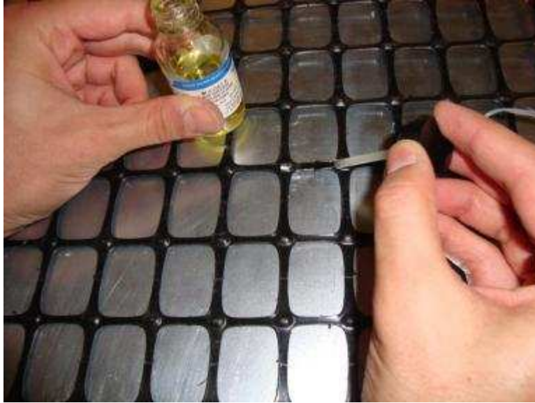
Figure 9.18. The gauge surface was covered with coating material
