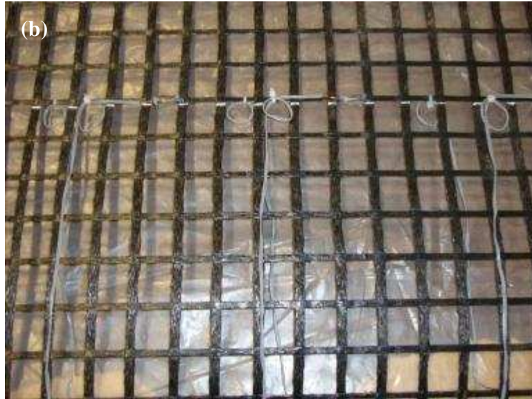
Figure 9.27. Example geogrid specimens instrumented with strain gauges: (a) EGG1, (b) WGG3
