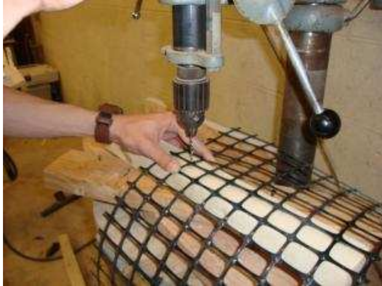
Figure 8.4. Drilling of the geogrid junctions to connect the extensometers
