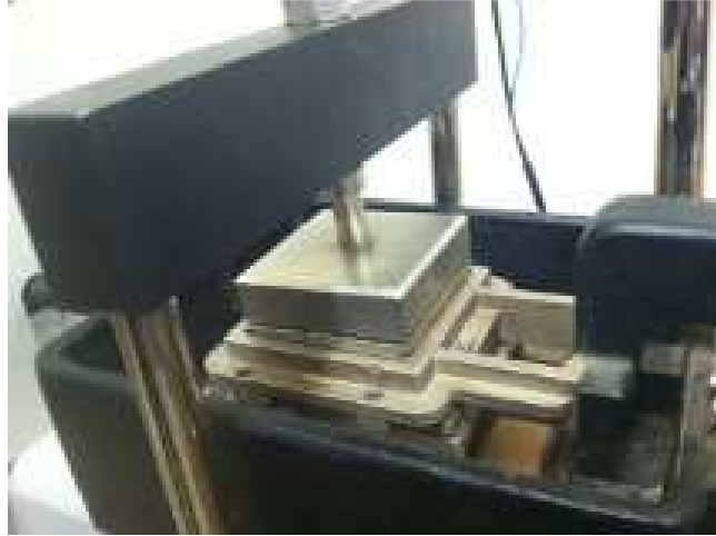
Figure 6.5. Final setup of the test cell the DST machine
