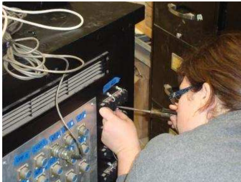
Figure 9.43. Connecting strain gauges to the DAS (Data Acquisition System)
