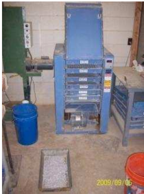
Figure 6.1. Sieve analysis equipment at the OU Broce Laboratory
