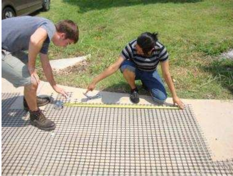
Figure 7.2. Geogrid sample preparation
