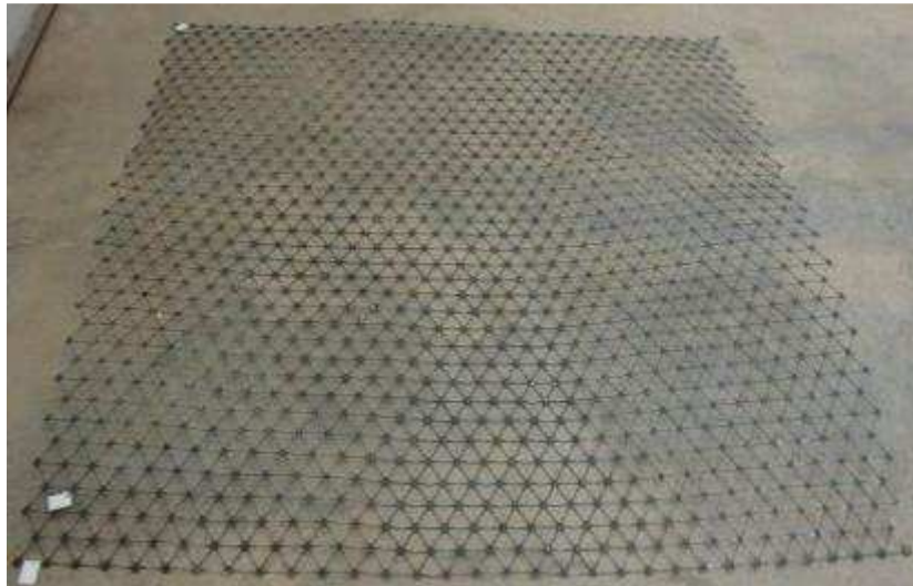
Figure 9.63. EGG4 geogrid specimen after the cyclic plate load test
