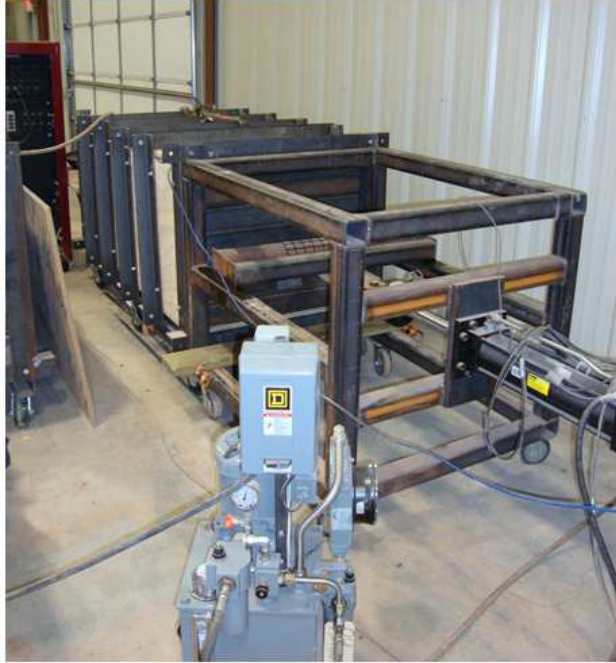
Figure 8.14. Completed pullout test setup before the test
