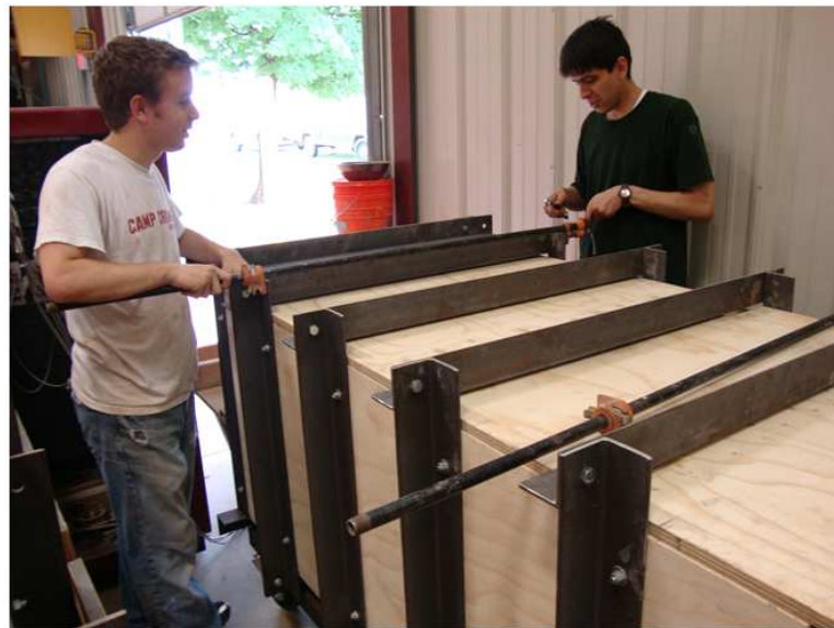
Figure 8.11. Closing of the pullout test box before the test
