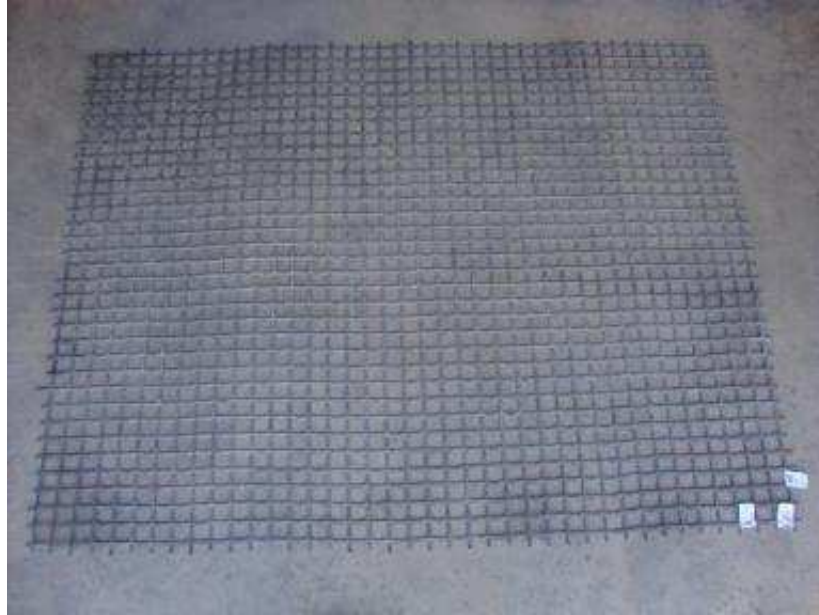
Figure 7.40. WGG3 geogrid specimen after exhumation
