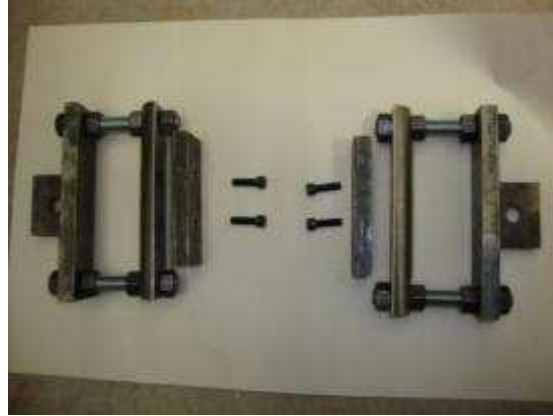
Figure 5.8. Clamping system fabricated to test non-extruded geogrids
