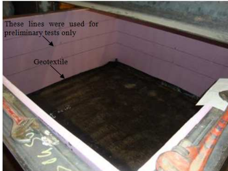
Figure 9.31. Cyclic plate load test box after placing the geotextile separator on Styrofoam panels on the bottom of the test box
