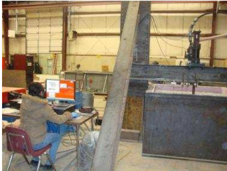
Figure 9.8. Cyclic loading tests on reinforced base-substrate models using the new controller system
