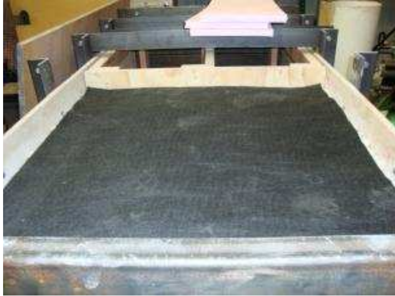
Figure 8.8. A separator geotextile was placed on the top of the aggregate
