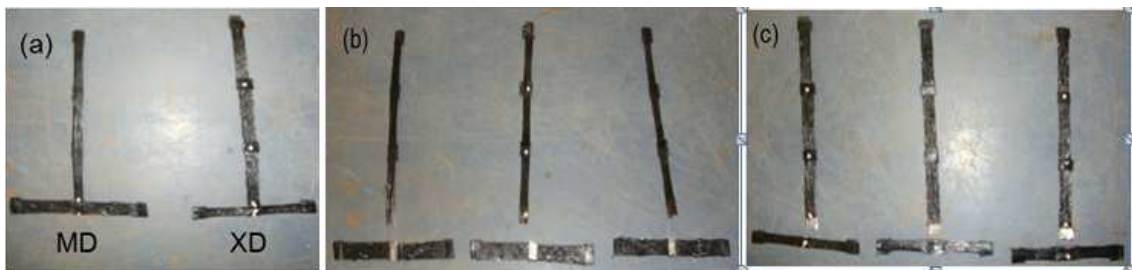
Figure 4.11. WGG3 geogrid junction strength specimens (a) before the test, (b) after failure (MD), (c) after failure (XD)
