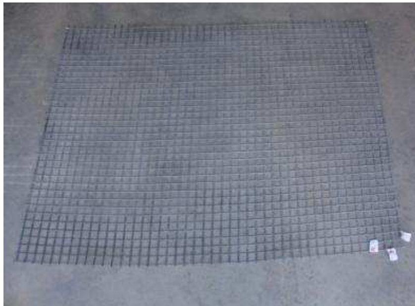
Figure 7.41. KGG1 geogrid specimen after exhumation
