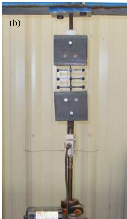
Figure 5.3. (a) Geogrid specimen secured in the clamps, (b) test setup mounted on the tension frame, (c) view from digital camera, ready to record the specimen deformation
