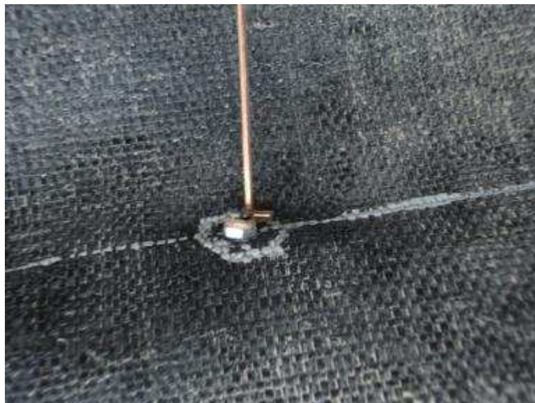
Figure 9.34. Attachment of brass wires to geotextile separator to measure its settlement
