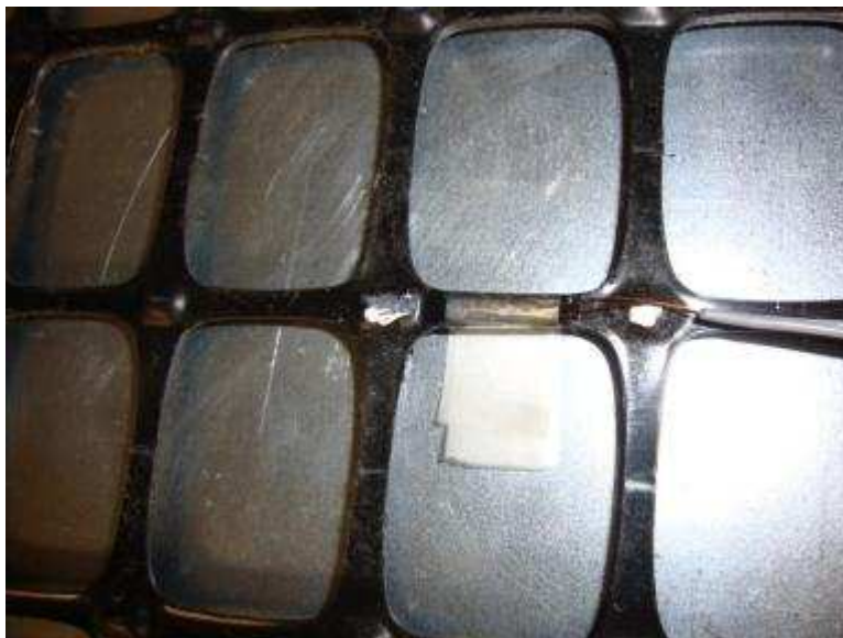
Figure 9.15. Gauges were held in place with the Scotch tape while the adhesive was cured
