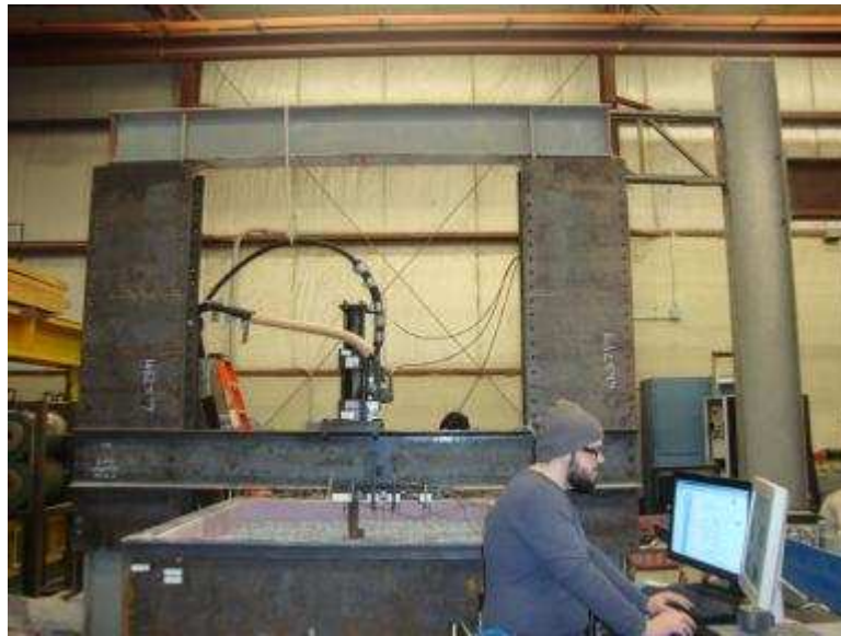
Figure 9.45. Monitoring data in the Data Acquisition System while a cyclic plate load test is in progress
