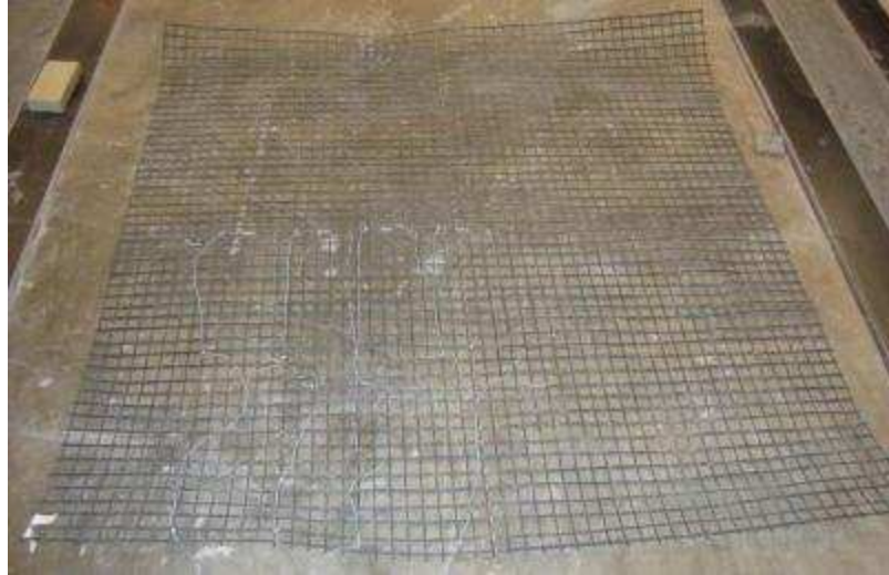
Figure 9.64. WGG1 geogrid specimen after the cyclic plate load test
