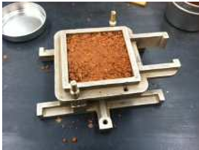
Figure 6.4. Dover sand in the test cell of the small-scale DST machine
