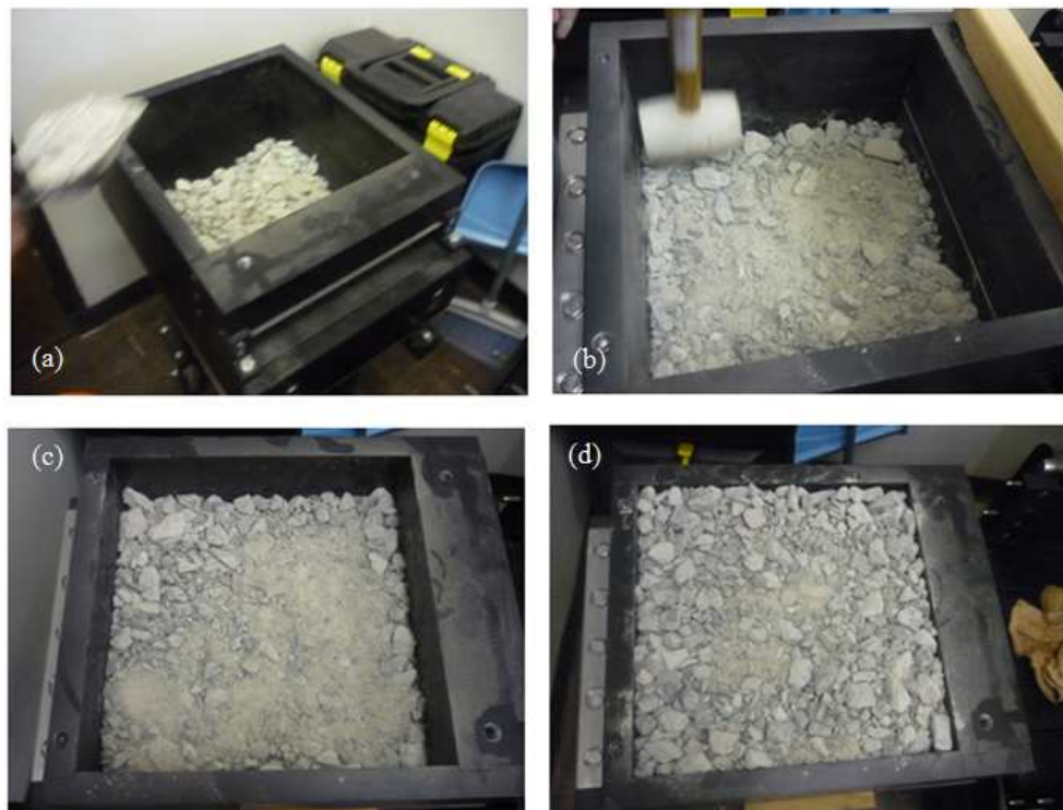
Figure 6.12. (a) Placing of first layer of aggregate in the shear box, (b) Compaction of first layer of aggregate with a mallet, (c) Second layer of aggregate after compaction, (d) Third (i.e. final) layer of aggregate after compaction
