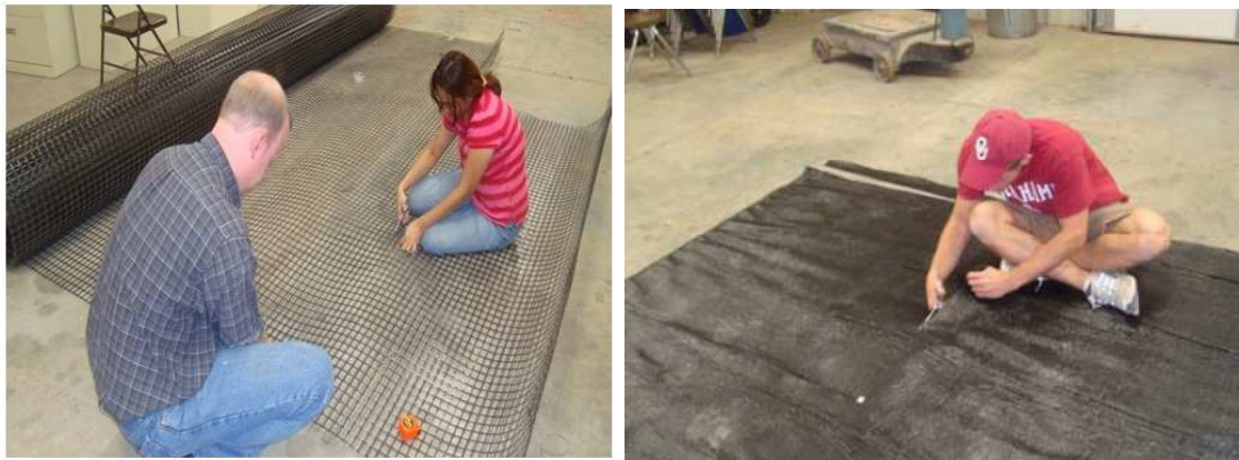
Figure 9.1. Preparation of the geogrid and geotextile specimen for a static plate load test
