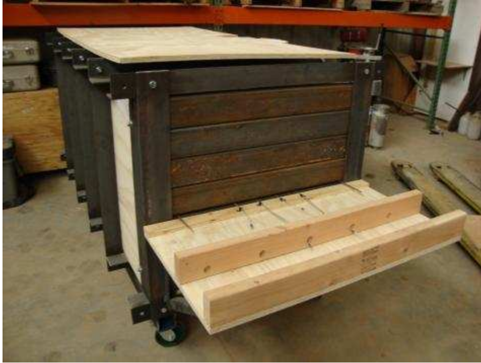
Figure 8.1. Newly fabricated pullout test box at the OU Fears laboratory
