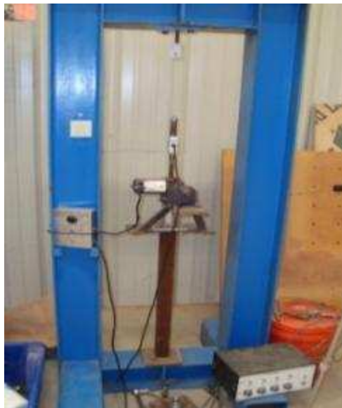
Figure 4.2. Tensile testing frame for testing rib and junction strength of geogrid specimens
