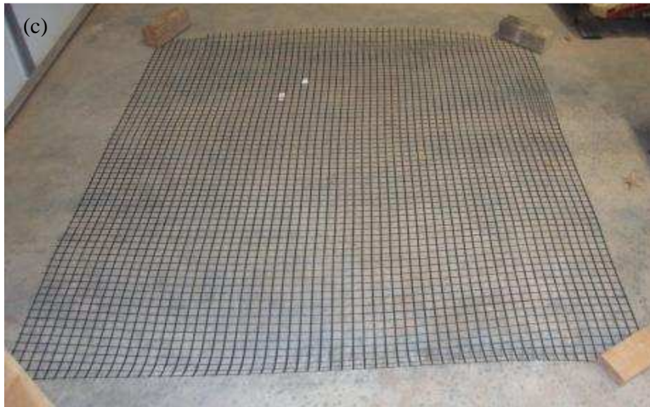
Figure 9.24. Geogrid specimen used in a cyclic plate load tests before instrumentation: (a) EGG1, (b) WGG1, (c) KGG1
