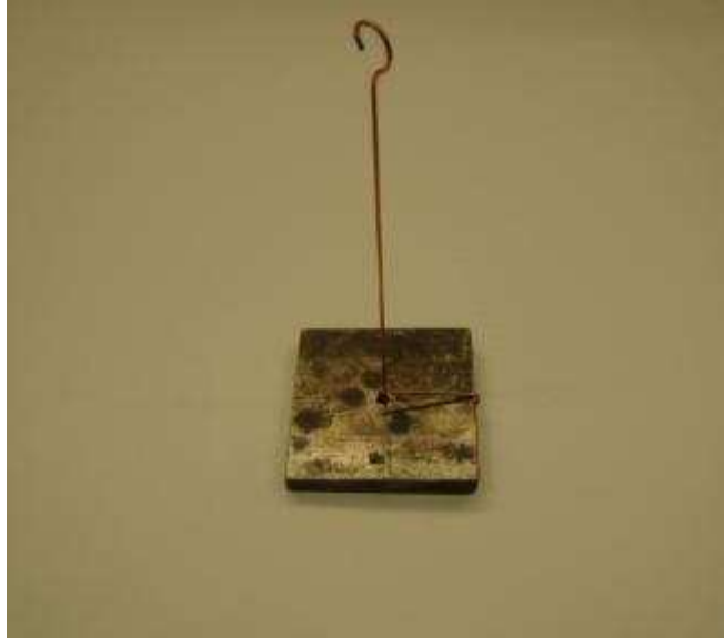
Figure 9.40. A telltale plate (50 mm × 50 mm) attached with brass wire to measure the surface deflection of the aggregate layer
