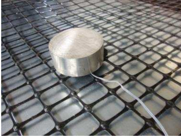
Figure 9.16. Pressure was applied to the gauge to cure
