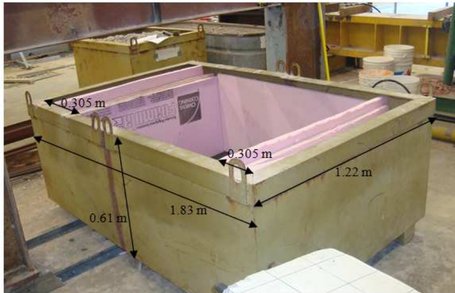
Figure 9.3. Test box used for the static plate load tests
