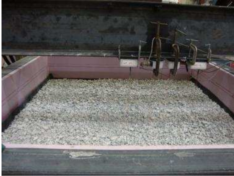
Figure 9.35. 25 mm-thick aggregate layer placed on the top of the geotextile separator
