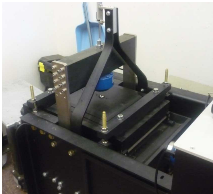
Figure 6.15. Large-scale direct shear test setup
