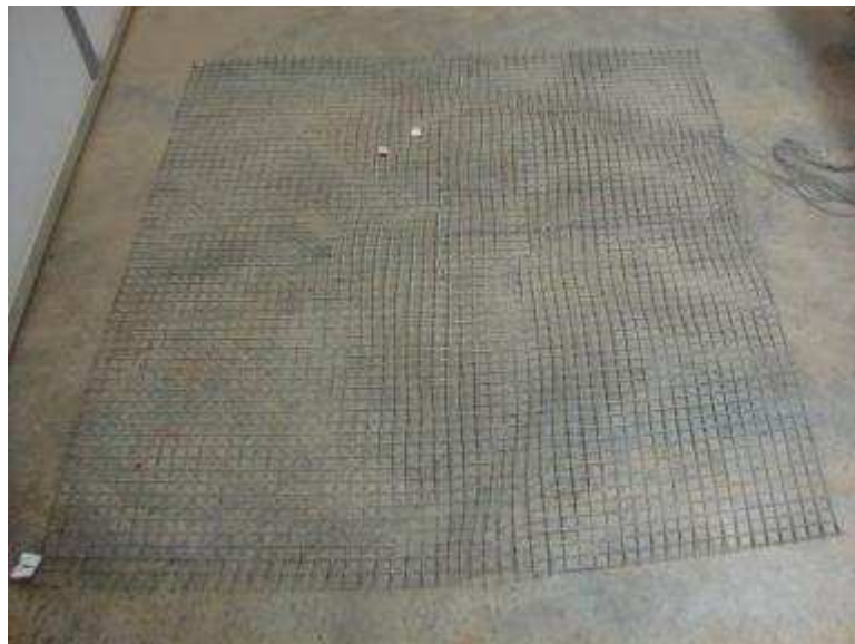
Figure 9.67. KGG1 geogrid specimen after the cyclic plate load test
