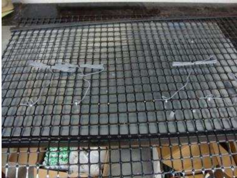
Figure 9.20. Geogrid with strain gauges attached
