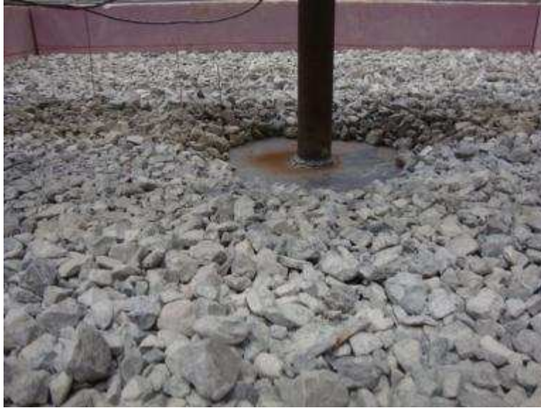
Figure 9.46. The position of the circular loading plate at the end of a test
