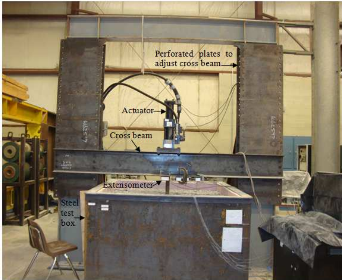
Figure 9.6. Redesigned and retrofitted steel loading frame at the Fears Laboratory
