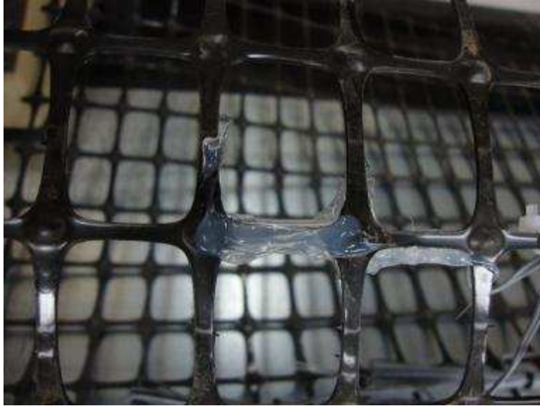
Figure 9.22. Siliocon rubber sealant was applied on the strain gauge
