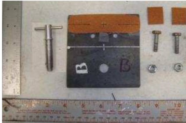
Figure 5.1. Rib strength test clamp for extruded geogrids and accessories
