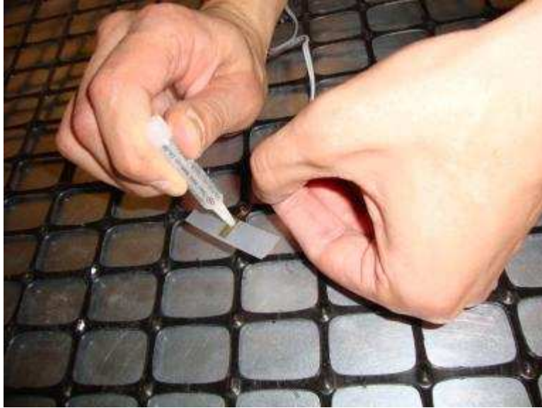
Figure 9.14. Application of adhesive material to the back of the strain gauge base
