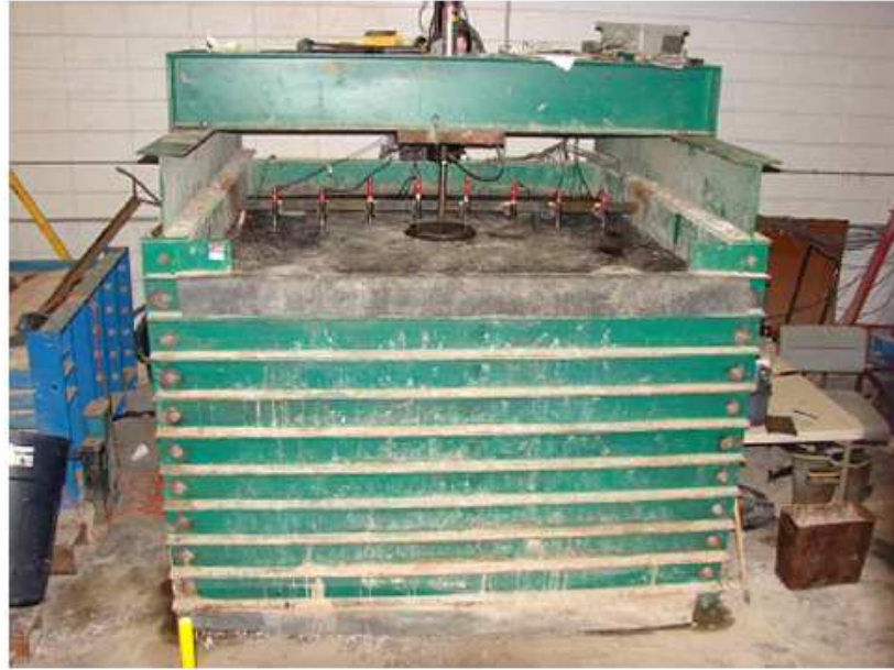
Figure 9.90. Laboratory test box, hydraulic actuator and reaction system in the study by Abu-Farsakh and Chen (2011)
