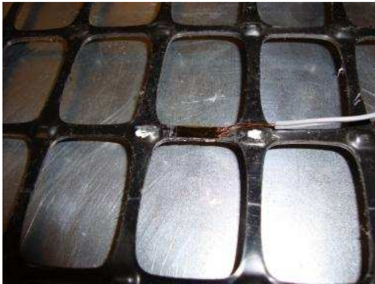
Figure 9.17. The tape was peeled off carefully from the strain gauge
