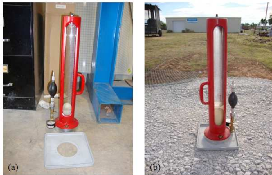
Figure 7.26. Measuring the in-situ density of aggregates (a) Model HM-310 Voluvessel Rubber Balloon densometer, (b) The densometer in use on the test bed
