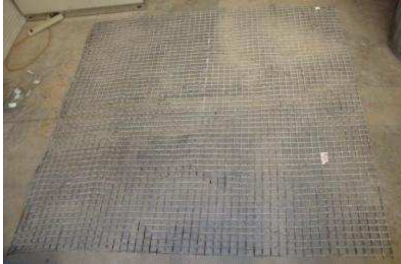
Figure 9.66. WGG3 geogrid specimen after the cyclic plate load test
