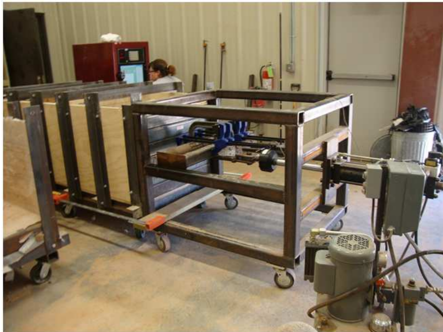
Figure 8.15. A pullout test in progress
