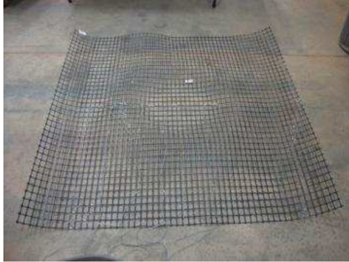
Figure 9.60. EGG1 geogrid specimen after the cyclic plate load test
