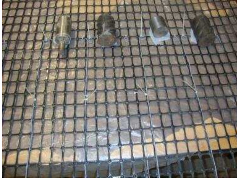
Figure 9.26. Pressure was applied to the gauges to cure their adhesive layer
