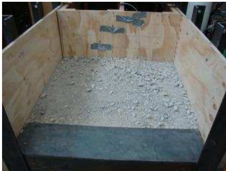
Figure 8.3. Compacted aggregate in the pullout box (the 203 mm-wide lower steel sleeve can be seen in the foreground)
