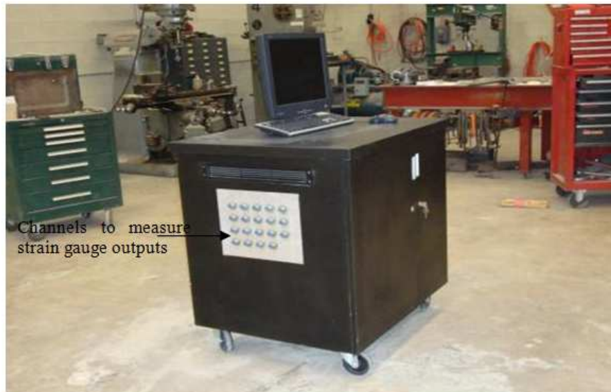
Figure 9.5. The new Data Acquisition System used in the cyclic plate load tests
