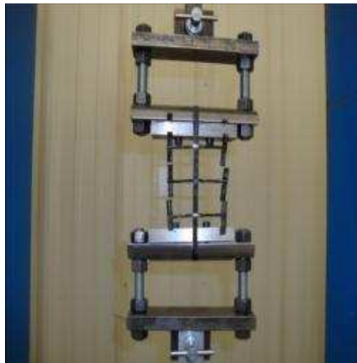
Figure 5.9. Rib strength testing of non-extruded geogrid in progress
