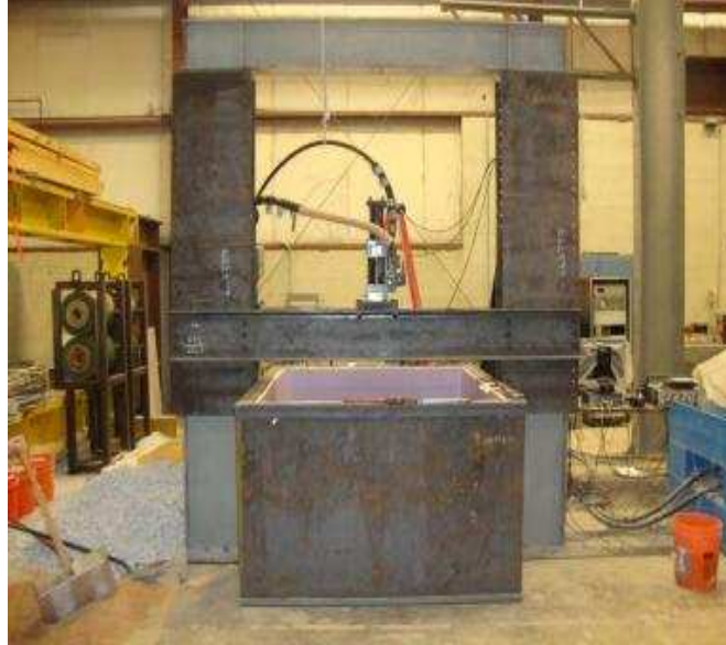
Figure 9.29. The redesigned and retrofitted steel loading frame with the actuator, which is connected to the hydraulic pump and the controller system
