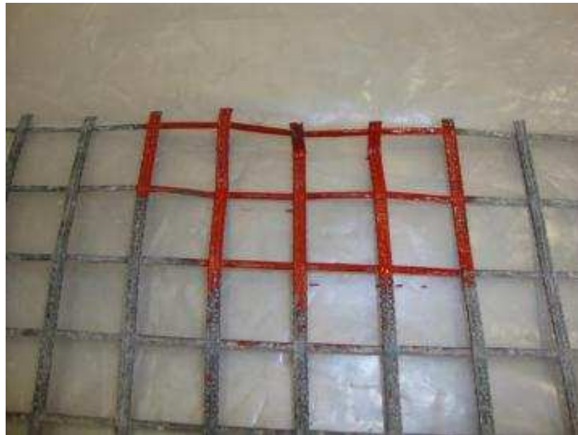
Figure 7.46. KGG1 geogrid sample with marked damaged area
