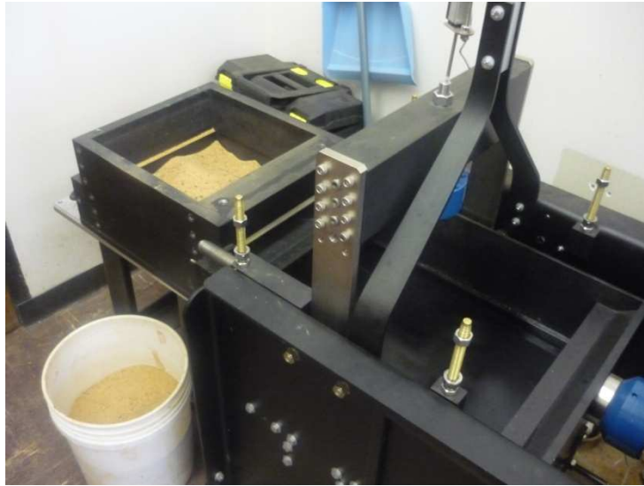
Figure 6.11. Setting up the large-scale DST machine to test sand specimens
