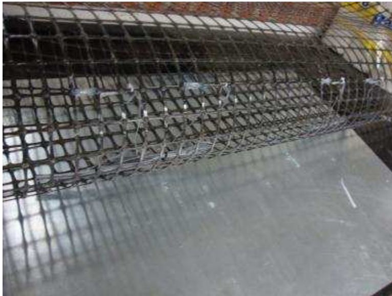
Figure 9.23. Geogrid sample left for 24 hours in order for the adhesive and sealant materials to dry out
