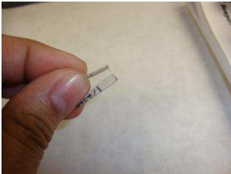
Figure 9.21. Flexible rubber tube was used to cover strain gauges
