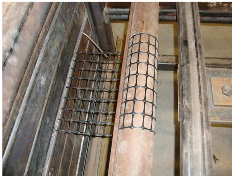
Figure 8.13. Geogrid attachment to the roller clamp
