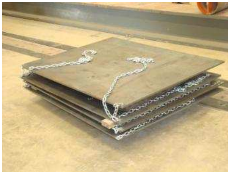
Figure 7.15. Steel plates with lifting chains
