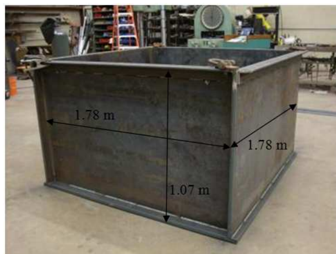
Figure 9.7. The newly fabricated large steel test box for cyclic plate load tests
