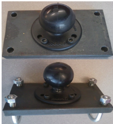
Figure B.6. Bracket used to attach the Tablet PC platform to the rail on the roller
