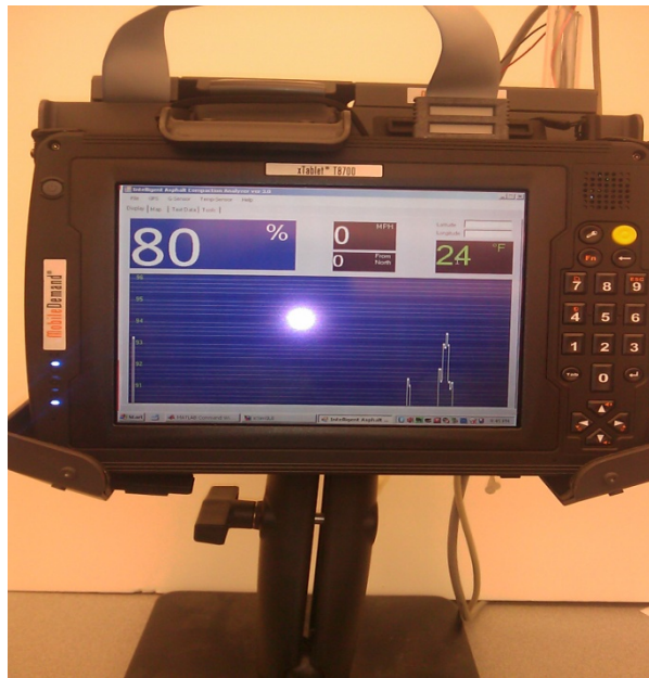
Figure B.1. T8700 Rugged Tablet PC with integrated numeric keypad (shown on mounting platform)
