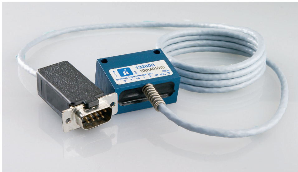
Figure B.4. Summit Instruments 10g uniaxial accelerometer
