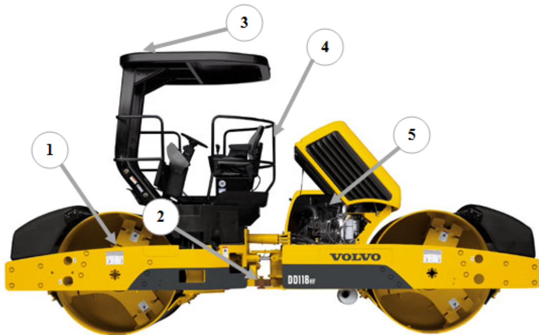
Figure B.8. Mounting location labels on a Volvo DD118HF roller.
