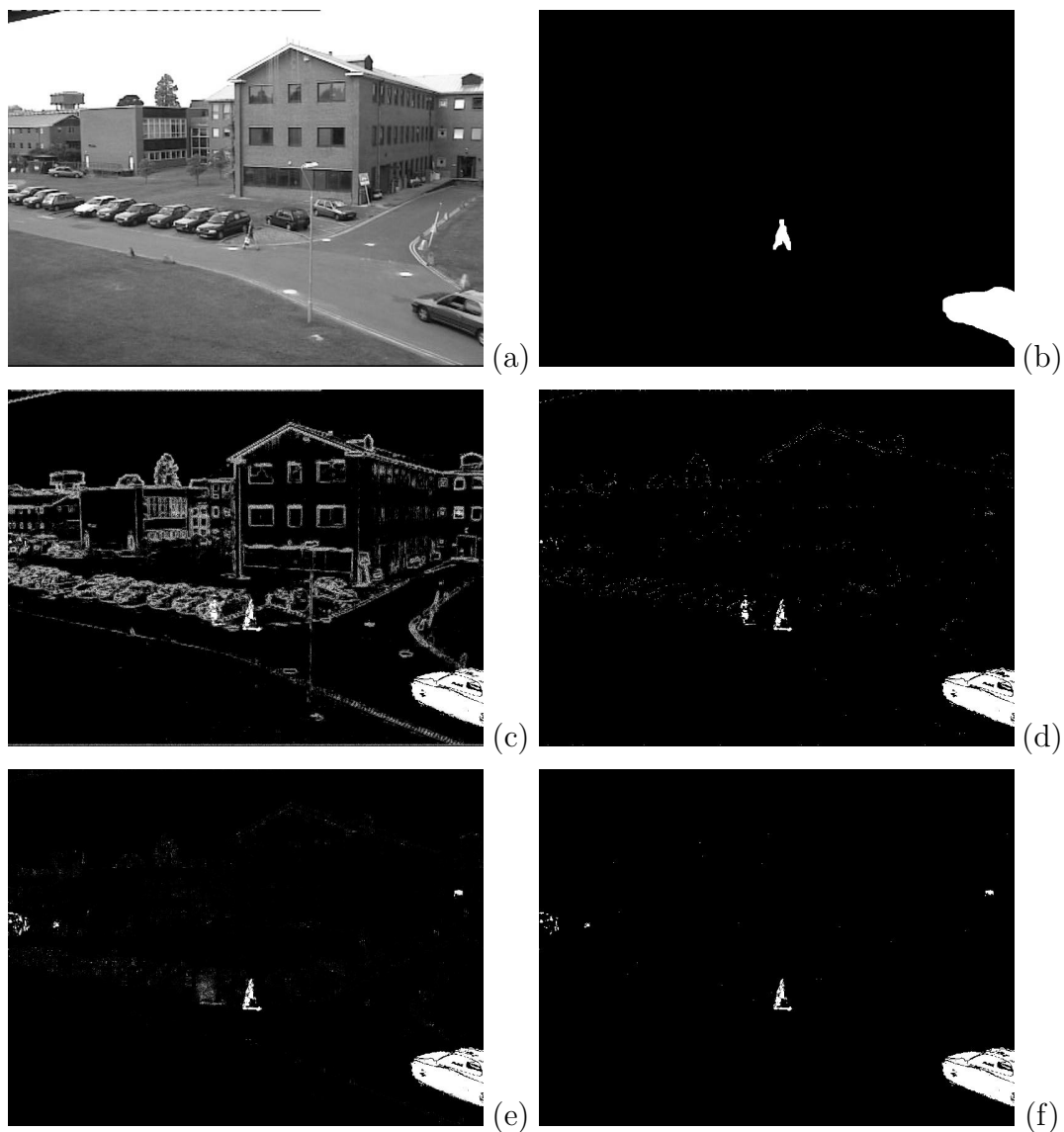
Figure 4.24: Frame 475 of the PETS 1 sequence depicting the original grayscale image (a), manually generated ground truth image (b), ViBe foreground probability image (PrCC=92.96%)(c), ViBe final segmentation (PCC=99.19%)(d), the foreground probability image for the proposed algorithm (PrCC=99.02%)(e), and the final segmentation for the proposed algorithm (PCC=99.40%)(f).
