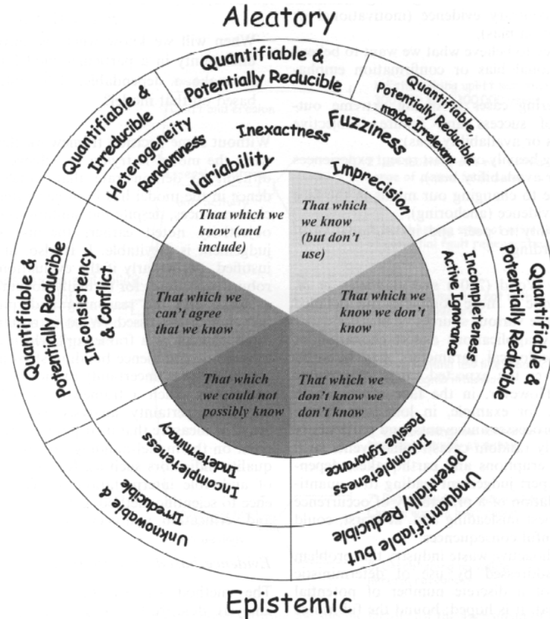
Figure E.1: Types of uncertainty can be classified as Aleatory (system variability) and Epistemic (lack of knowledge), all of which can be found in a typical wellbore stability analysis (from Bowden, 2004). While the aleatory uncertainties can be identified and quantified as probability functions, epistemic uncertainties are most often subjected to human biases.
