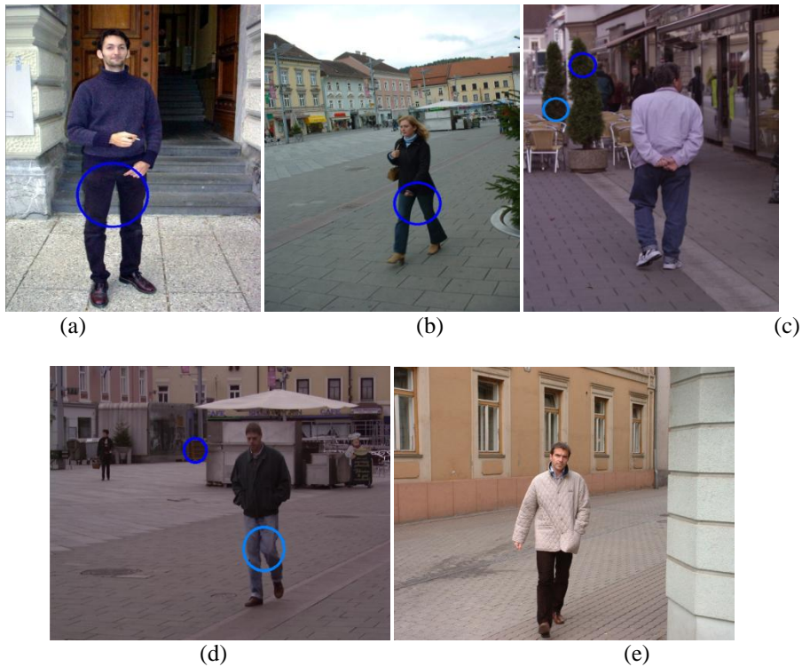
Figure 2.6 – Haar-like legs detector trained with 890 samples, (a) & (b) complete detection, (c) no detection and false positive, (d) detection with false positive, and (e) no detection.
