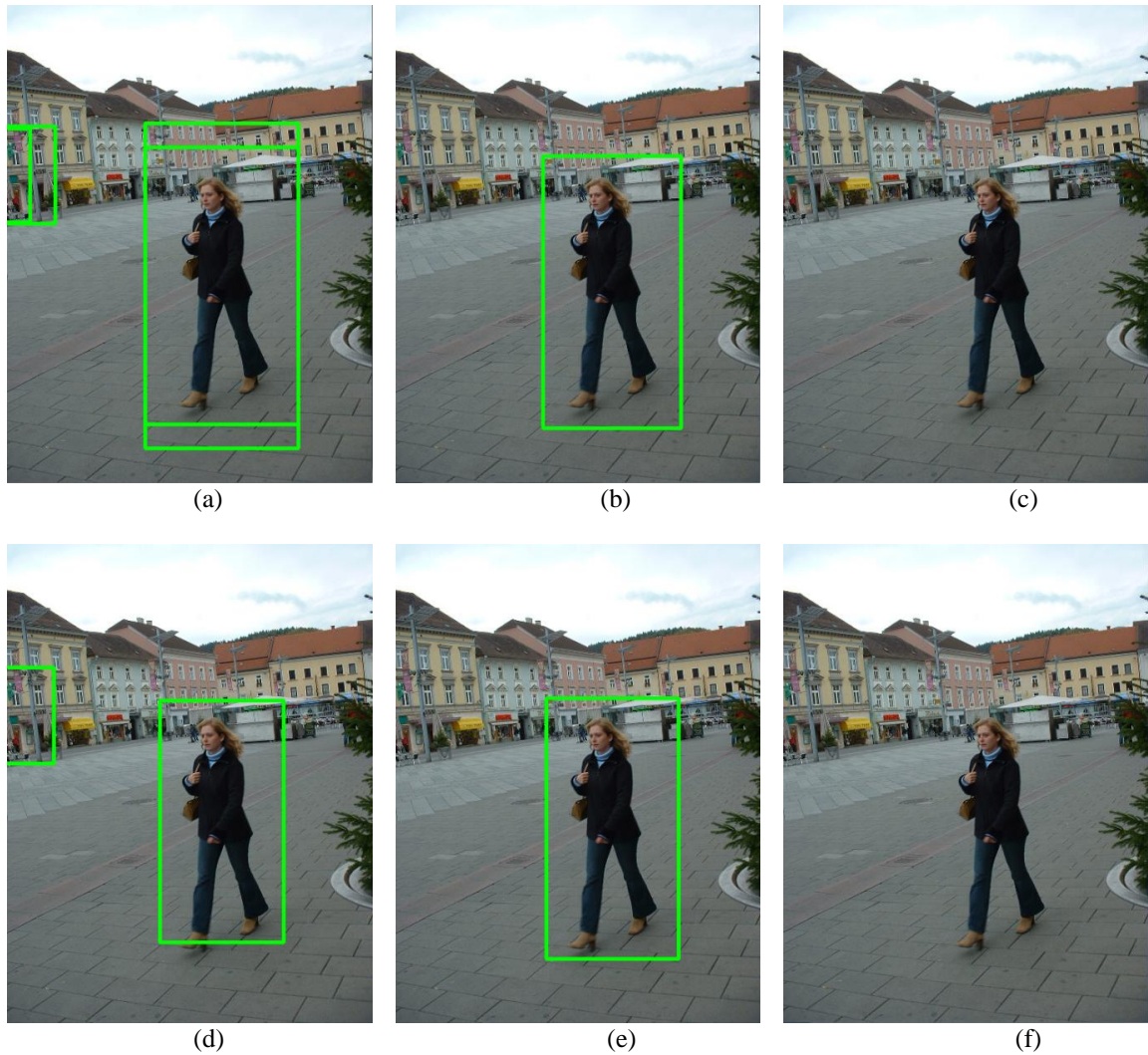
Figure 3.5 – Varying the hit threshold value in HOG human detection: (a) ht = 0 and gt = 0 , (b) ht = 1 and gt = 0 , (c) ht = 2 and gt = 0 , (d) ht = 0 and gt = 1 , (e) ht = 1 and gt = 1 , (f) ht = 2 and gt = 1 .
