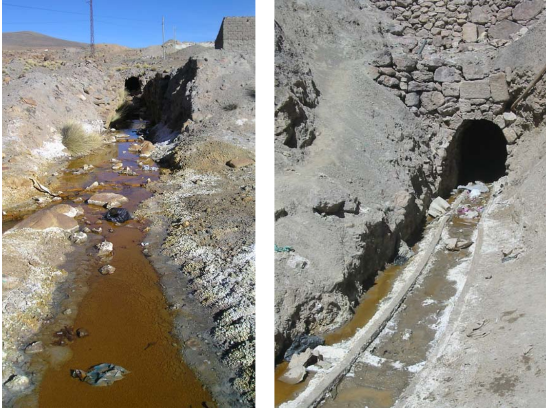
Figure 2.2 AMD sources 1A (left) and 1C (right). Source 1A is an abandoned portal near the eastern base of Cerro Rico. Source 1C is a functioning mine portal on the north slope of Cerro Rico.
