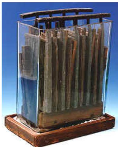
*Figure 1.4 Lead-Acid Cell (Figure reproduced from [http://en.wikipedia.org/wiki/History\\_of\\_the\\_battery](http://en.wikipedia.org/wiki/History_of_the_battery))*
