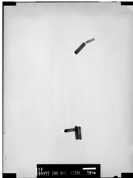
Figure 5.13. TEM image of gold nanorods with average AR of 3.8 (see Figure 5.10 for absorption spectrum).
