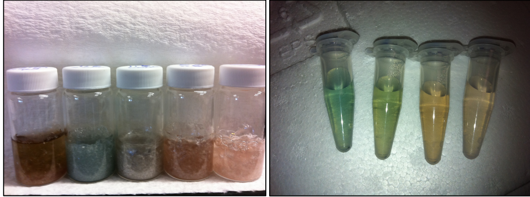
Figure 5.11. (left) Reaction vials of gold nanorod preparation: Seed solution (brown) 40-90 \mu\text{L} of silver nitrate added (respectively); (right) GNR 40-90 \mu\text{L} (respectively) with excess CTAB (white crystals seen left) removed via centrifugation.
