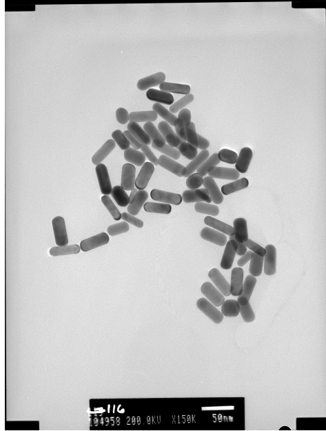
Figure 5.12. TEM image of gold nanorods with average AR of 2.7 (see Figure 5.10 for absorption spectrum).
