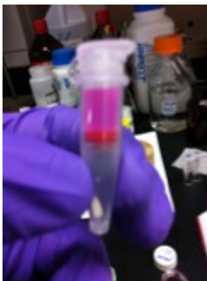
Figure 2.24. Nanosep centrifugal device prior to be centrifuged. The red band is a label for the MWCO (30 kD)
