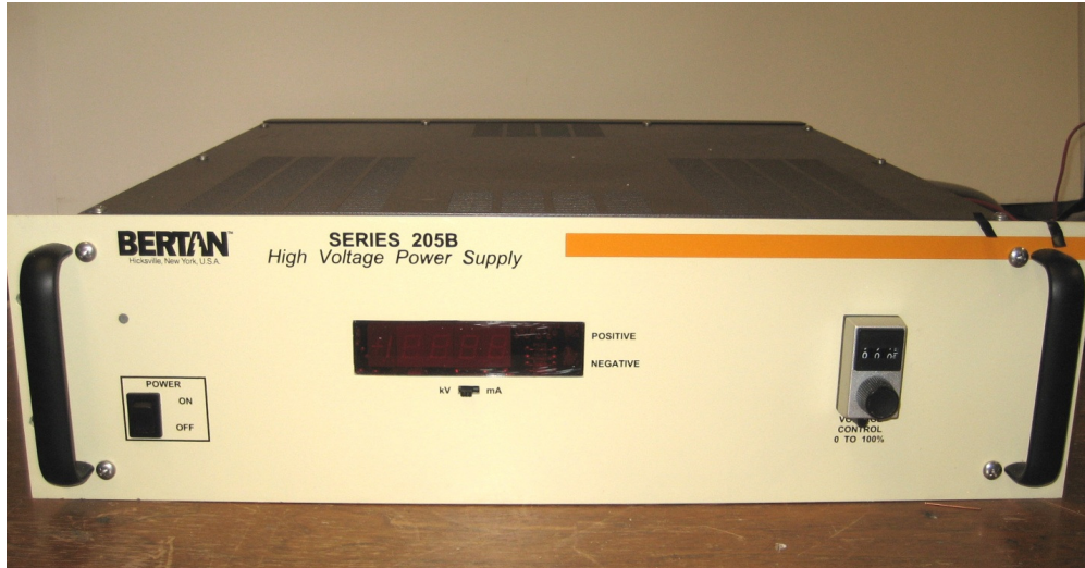
Figure 2.3 High voltage power supply
