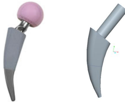
Figure 3-11: (a) “Metha Short Hip System” Hip-replacement joint, (b) Similar Hip-replacement joint created by the grammar
