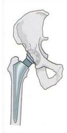
Figure 5-5: A total hip replacement inserted into a human femur and hip (Hamrock et al., 2005)
