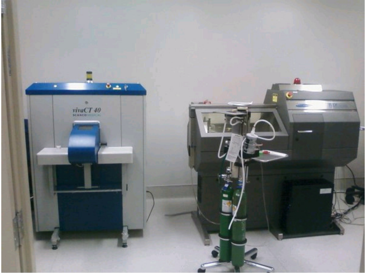
Figure 3 ScanCo VivaCT40 (ScanCo Medical, Bassersdorf, Switzerland; http://www.scanco.ch ) used in this study is shown on the left side.
