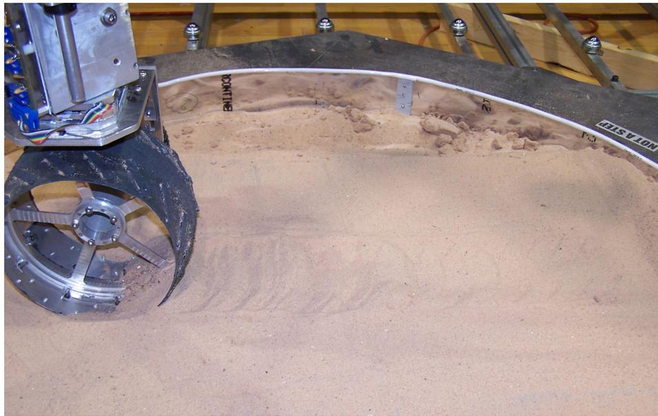
Figure 9.4: Painted wheel mounted on SWEET pulling load in sand
