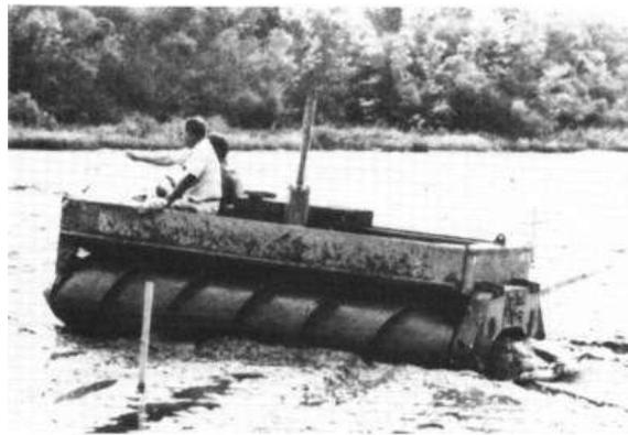
Figure 4.10: Chrysler Marsh Screw Amphibian [2]
