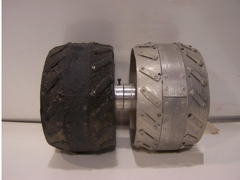
Figure 9.1: Metal rover wheels, right bare wheel used on SR2 rover [61]. Left wheel is painted with Herculiner [39] high friction paint.
