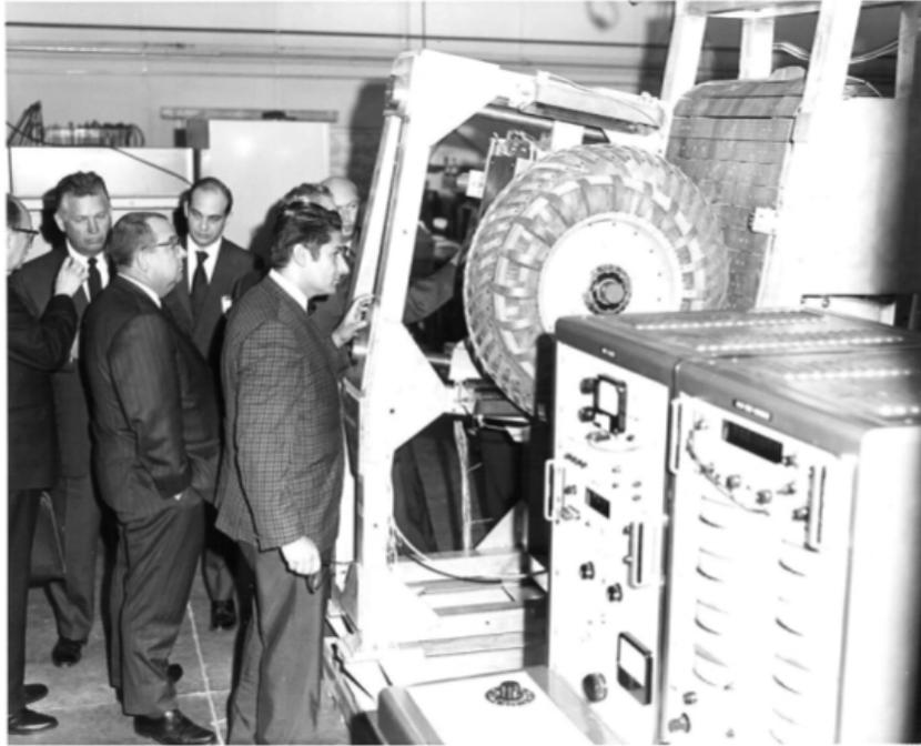
Figure 2.21: GM Testbed for LRV Wheel [71]
