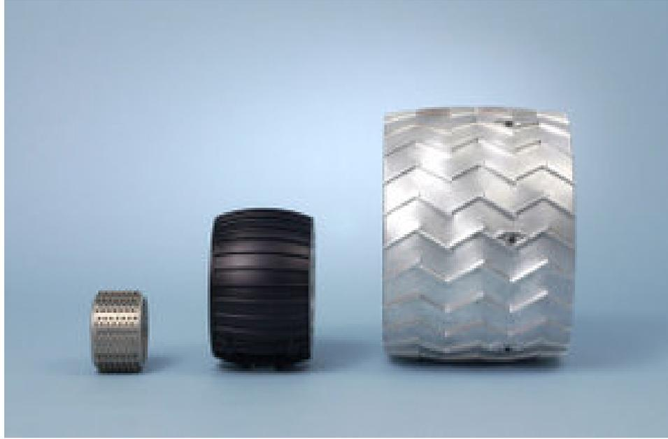
Figure 2.11: Wheels from Sojourner (left) MER (center) and MSL (right) *image by NASA*
