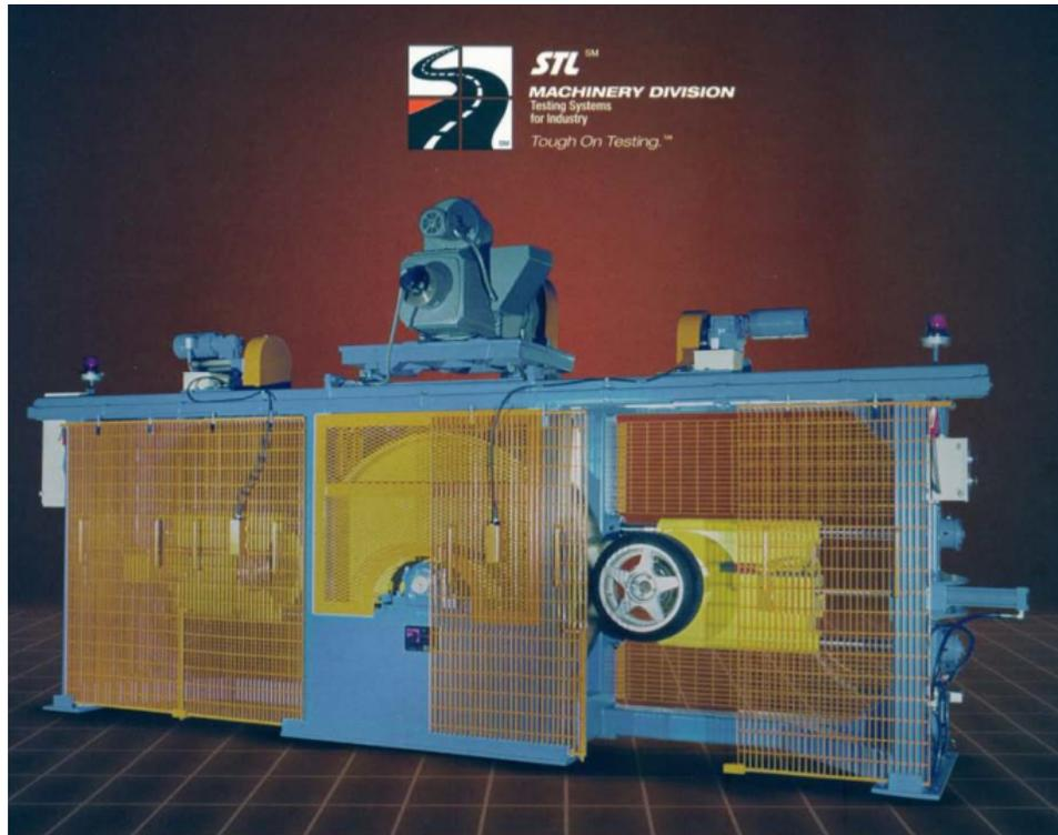
Figure 2.28: STL Radial Fatigue Test Apparatus [66]
