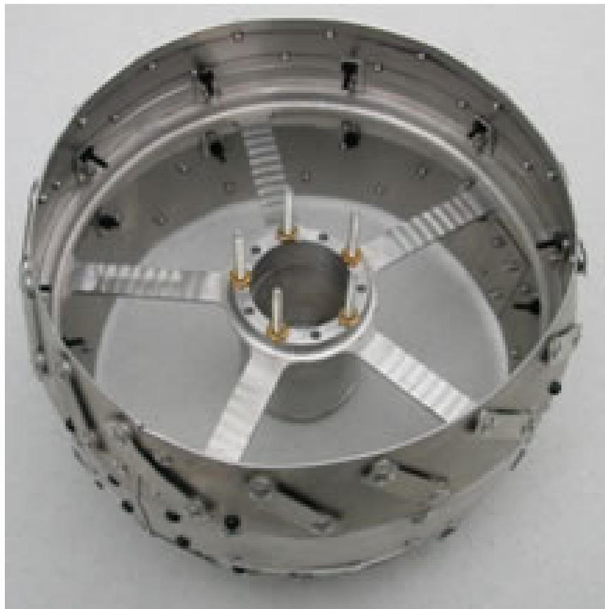
Figure 4.16: SR2 chamfered wheel with side mounted grousers
