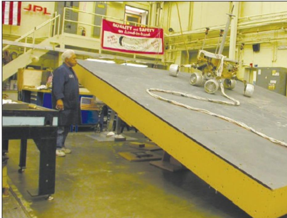
A Model Robotic Vehicle was driven over 25-cm obstacles on simulated terrain at a tilt of 20°.
