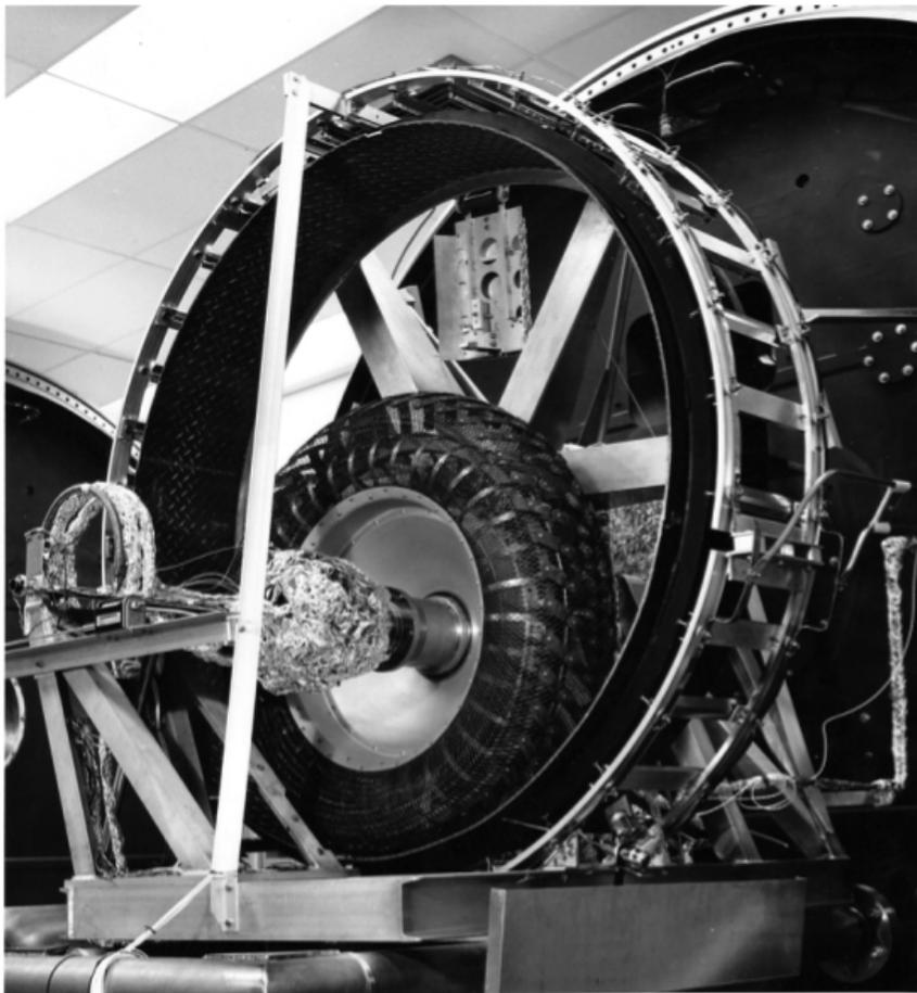
Figure 2.20: GM Testbed for LRV Wheel [71]
