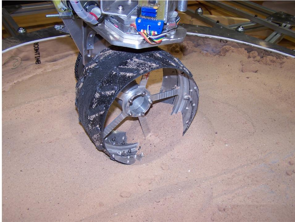
Figure 9.3: Painted wheel mounted on SWEET in static friction test on sand
