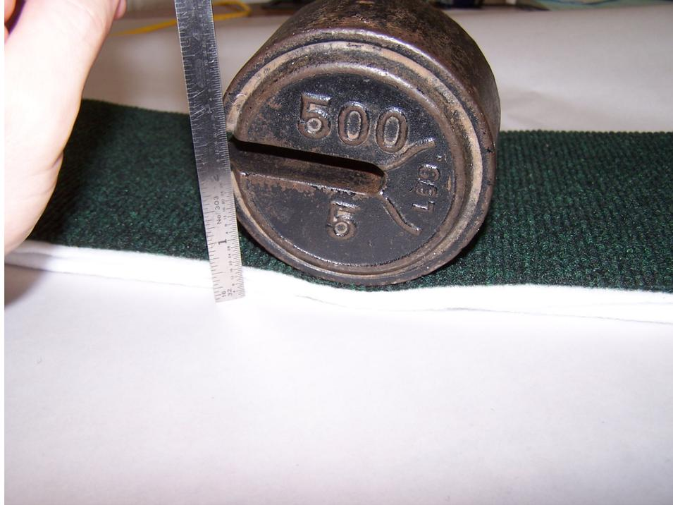
Figure 7.2: Padded test carpet surface with 5 lb weight
