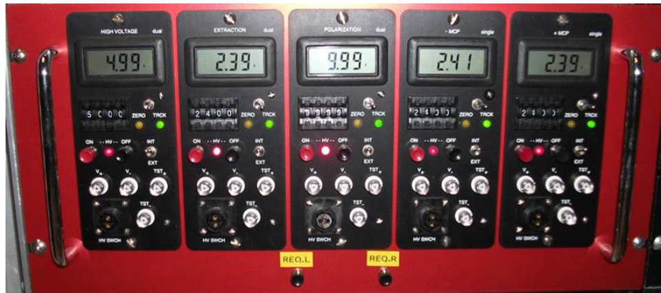
Figure 3.2: The front panel of the high voltage control unit. Numbers appear in displays are in kV
