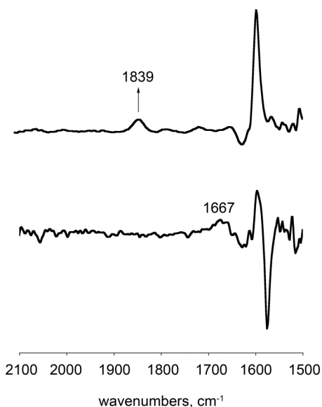
Figure 4.20. Difference IR spectra showing the products from the first oxidation of the (T( p -OMe)PP)Fe(SalHate) compound containing 0.1 M NBu 4 PF 6 with potentials held near the E_{pa} of the first oxidation (top) and with a proton sponge (bottom).
