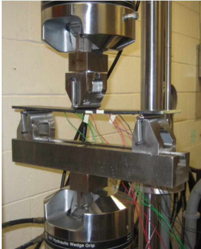
Figure 6.5 Test setup for 3-point bending in the MTS
