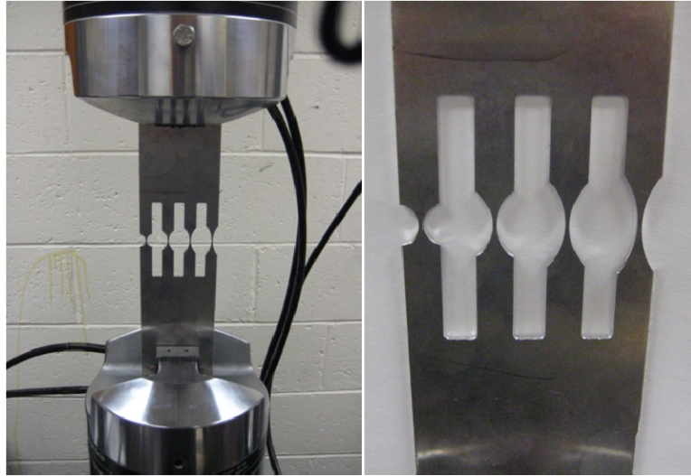
Figure 4.5 Test setup and specimen design utilized in the proof-of-concept experiment (Wijesinghe 2010)
