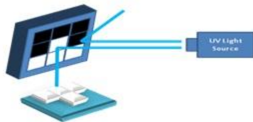
Figure 3.3 Representation of Digital Micro-mirror Device. The middle row shows the “on” mode micro-mirrors.
