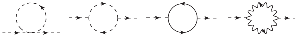
Figure 3.1: Radiative Correction to the Mass of Scalar Higgs. The first two loops come from the contributions of Higgs boson respectively through the interaction of four Higgs bosons and the interaction of three Higgs bosons. The third denotes the contribution from fermion while the fourth is for the gauge bosons.
