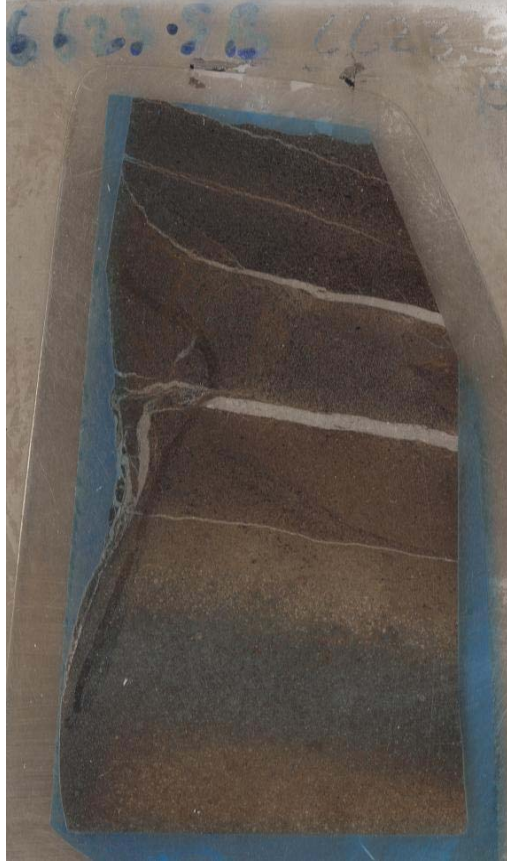
Figure 2-26. ASW 6623. bedding parallel or stratiform fractures. Discolored bed below contains bedded pyrite and phosphate. Note the transition to sub-vertical fracture (northeast azimuth) on the left side of the photo suggesting a possible genetic relationship between the two fracture types. Sample is 2.3cm wide.
