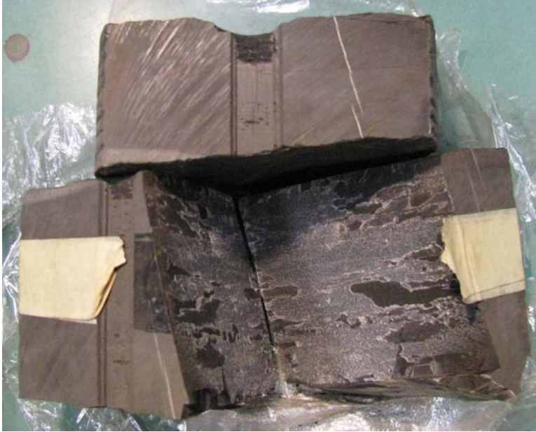
Figure 2-32. An exposed partially healed en echelon fracture, northwesterly, ES core. Note the fracture plane shows a incomplete distribution of cement. Core is 4” in diameter.
