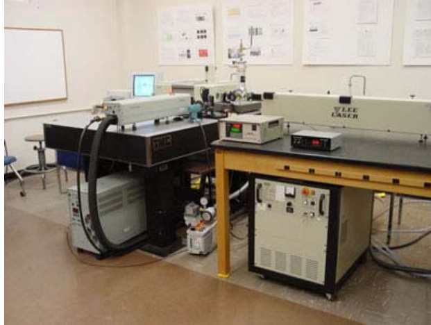
Fig. 3.15: Bruker IFS66/S FTIR measurement system in OU optical lab.
