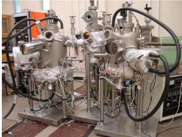
Fig. 3.7: Custom designed MBE growth chamber in opto-electronics lab at OU.
