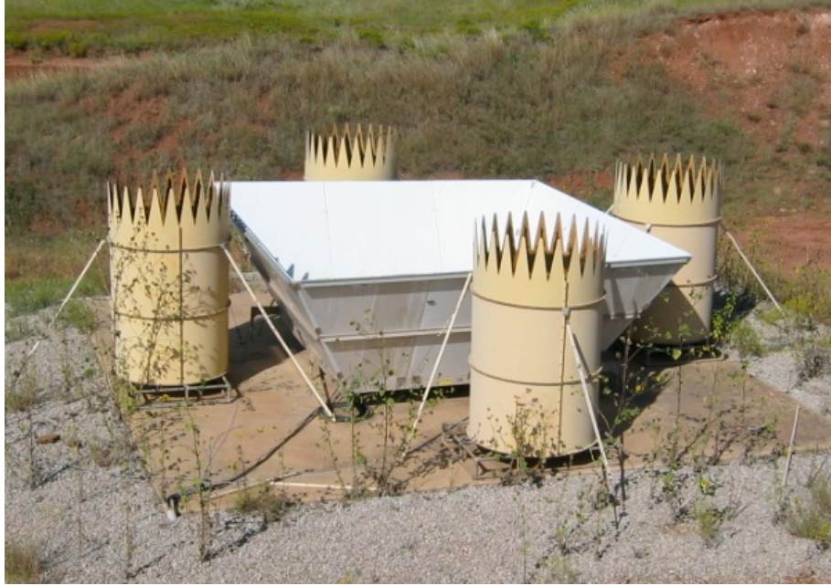
Figure 4.1: Picture of the Radial Wind Profiler (RWP) located at the SGP ACRF. In addition to the wind profiles, the system can obtain virtual temperatures through the Radio Acoustic Sounding System (RASS) co-located with the radar (Courtesy of Dr. P. Chilson).
