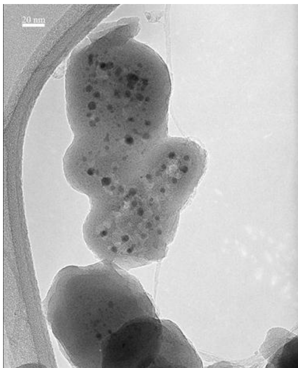
Figure 46(b): TEM image of SWCNT grown onto Co-Mo/SiO 2 powder catalyst with NH 4 OH/TEOS ratio of 6/6.
