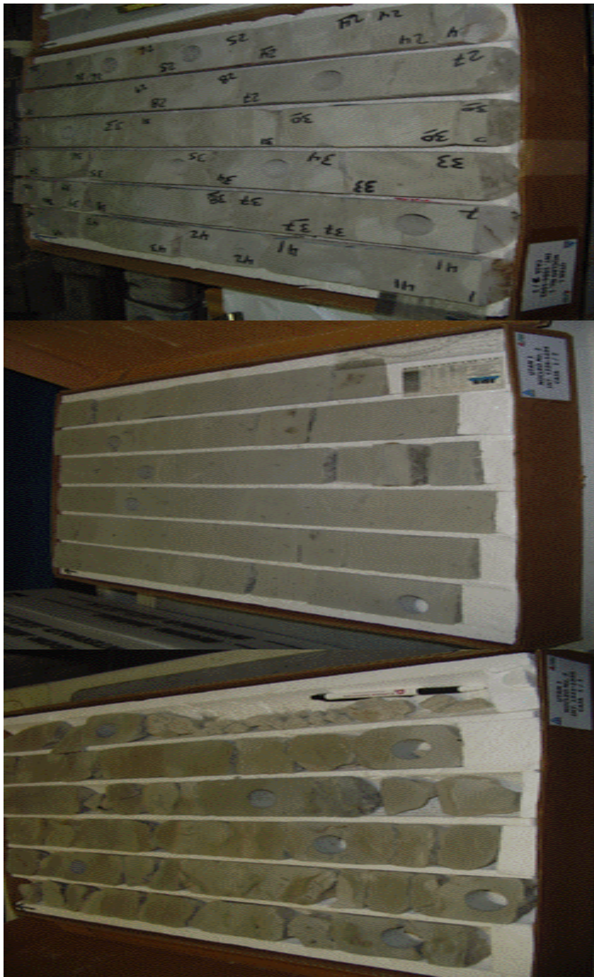
Figure 6.4: After the comprehensive detailed visual analysis, it was concluded that all three cores of the Utan well exhibited similarities and a general mixed calcareous-siliciclastic lithology. (Upper) Core 3 (1084-1092.5m); (Middle) Core 2 (1225-1232m); (Lower) (1321-1324.4).
