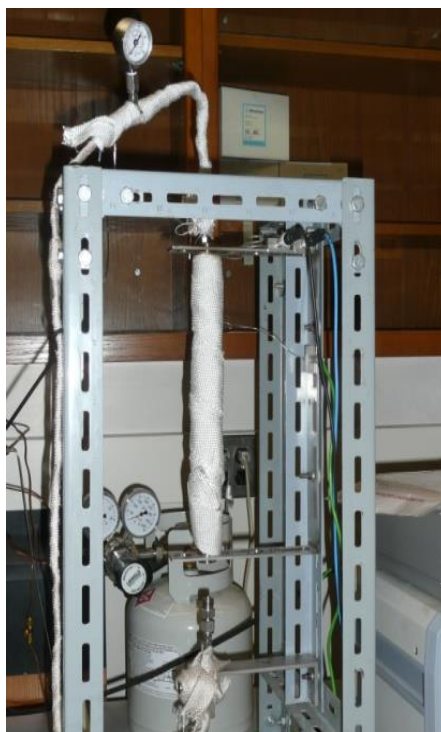
Figure 3.2: A picture of the furnace used to heat the packed bed apparatus.
