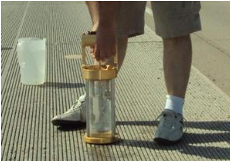
Figure 1.29 Outflow Meter Testing Apparatus
