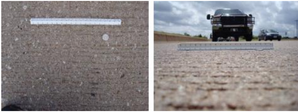
Figure 1.19 Test Section #15 – Shotblasting (Blastrac)
