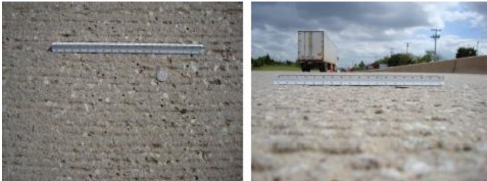
Figure 1.20 Test Section #16 – Shotblasting (Skidabrader)
