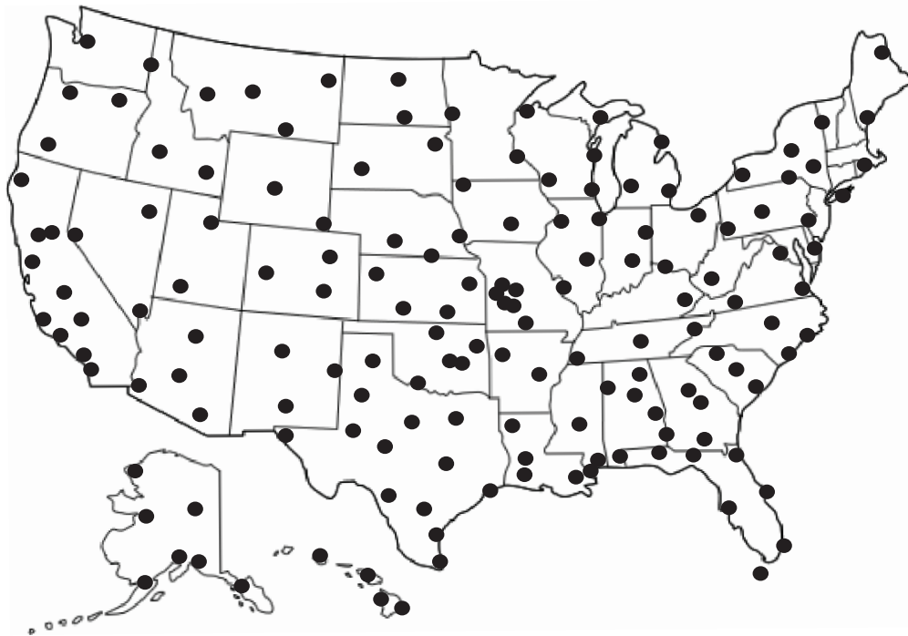
Figure 1.5: Distribution of radars operated by the NWS in 2009 ( roc.noaa.gov ). Located in all 50 states and consisting of 158 sensitive S-band Doppler radars, the current network operated by the National Weather Service aims to provide surveillance, forecasts, and warnings of all severe weather events.
