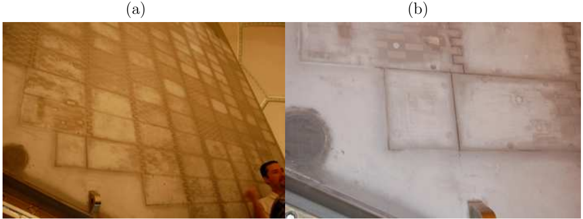
Figure 4.1: Images of SPY1-A antenna of NSSL PAR (courtesy of Boon-Leng Cheong). Shown are some examples of the receive subarray and sidelobe canceling modules of the NSSL PAR. These elements combine to form the antenna that is used for transmitting, receiving, and for mitigating clutter.
