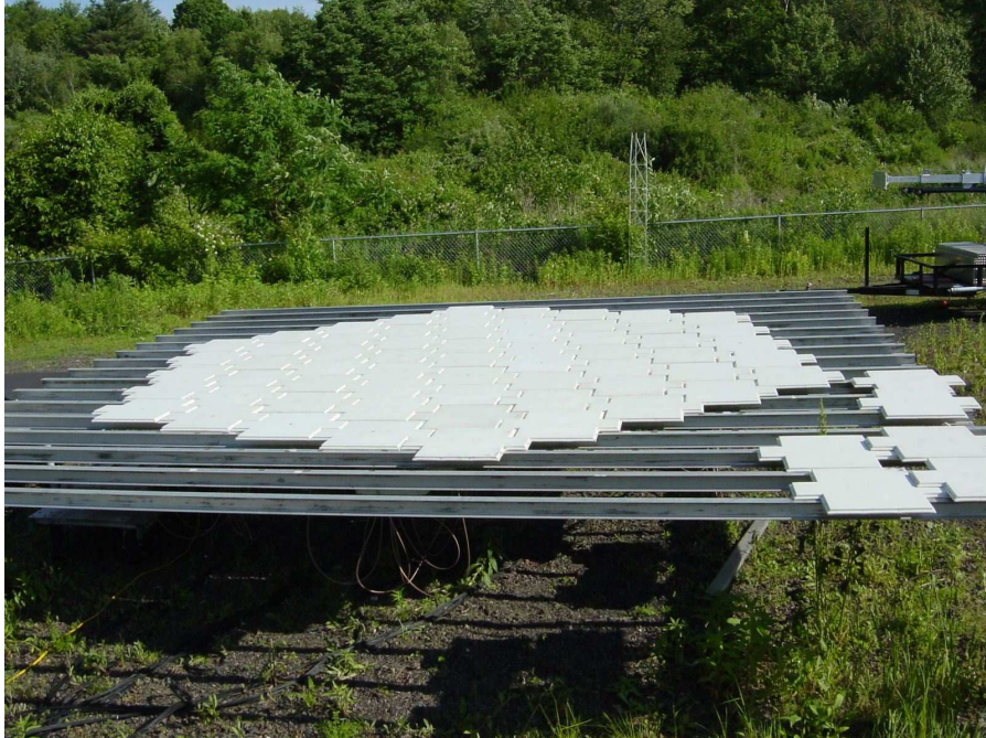
Figure 1.13: Turbulent Eddy Profiler (courtesy of Boon-Leng Cheong). This bistatic radar operated at 915 MHz and was used to investigate phenomena occurring in the boundary layer.
