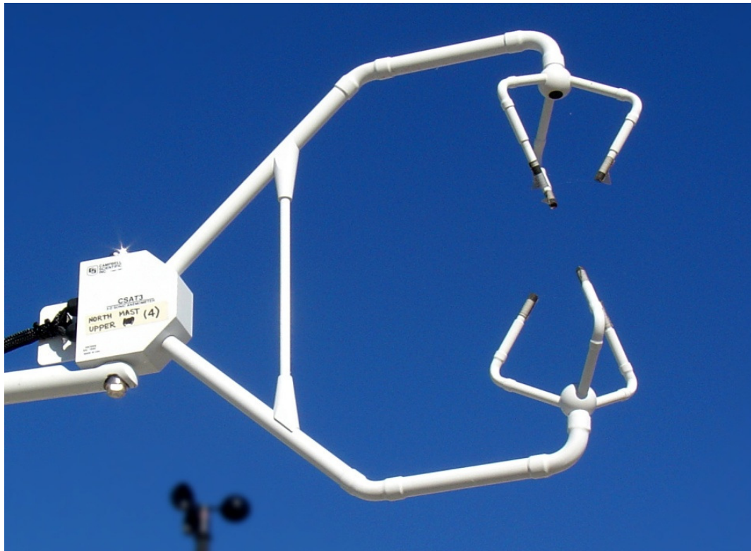
Figure 3.1. CSAT3 sonic anemometer. A cup anemometer can be seen in the background.
