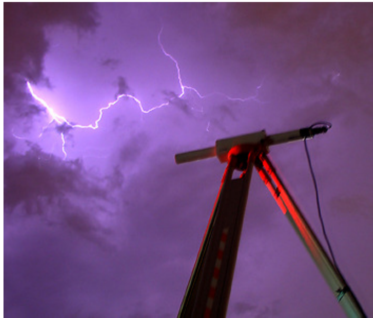
Figure 3.3. ILREUM SLS receiver during a lightning storm. April 2010.
