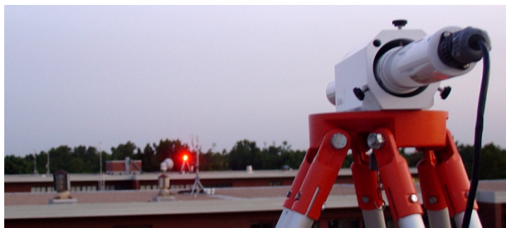
Figure 3.4. SLS transmitter (background) and receiver (foreground) collecting data during the core ILREUM campaign.
