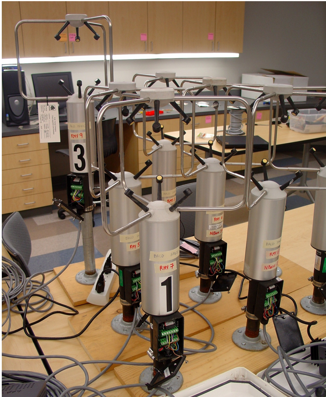
Figure 3.2. RMYoung sonic anemometers, Model 81000, being tested at the School of Meteorology (SoM - OU) Instrumentation Laboratory before the core ILREUM campaign.
