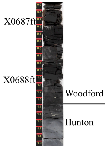
Figure 4.6-3: Core from well 1, showing the erosional unconformity between the Hunton Limestone and the overlying Woodford Shale.
