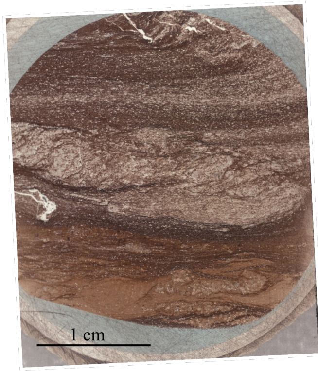
Figure 4.5-6: Slump visible at the high resolution scanned image of a thin section.
