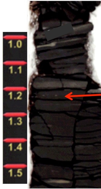
Figure 4.6-5: A section of core showing the contact at X0555 ft in well 1 (marked by red arrow).
