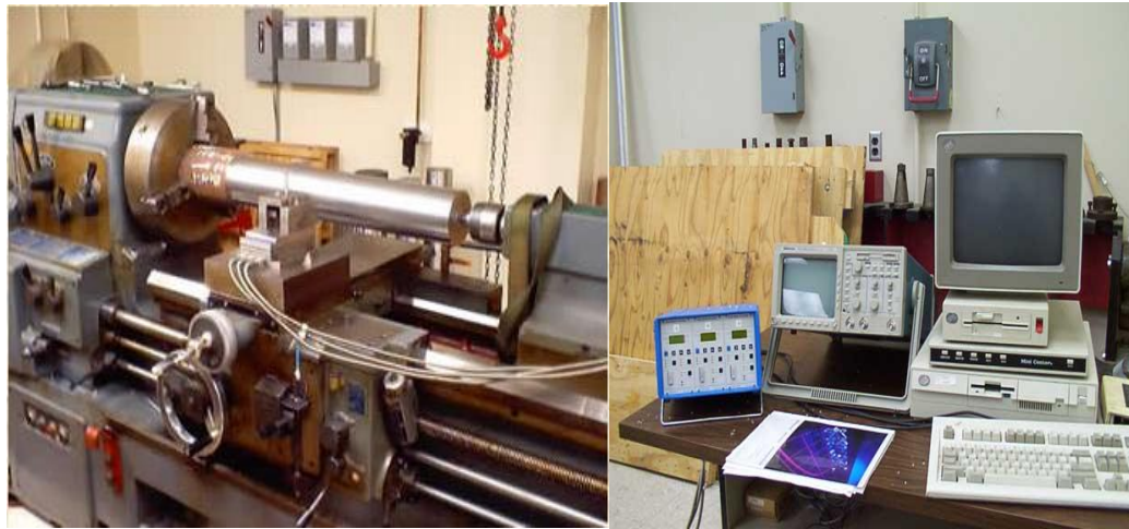
Figure 3.1. Industrial lathe and data acquisition system
