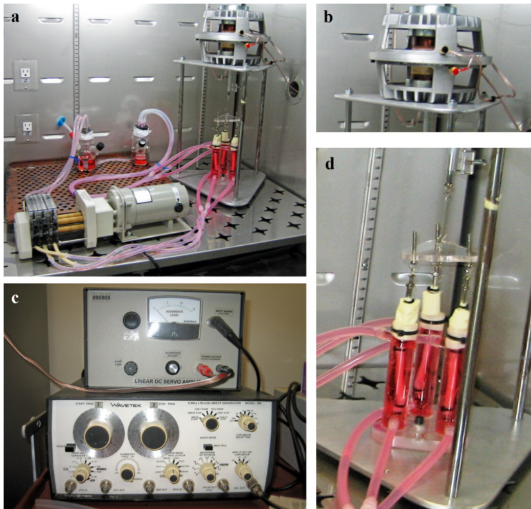
Figure 5.1: (a) Design of the Bioreactor, (b) Linear Motor, (c) Amplifier and signal converter, and (d) Close up to the reactor vessels.
