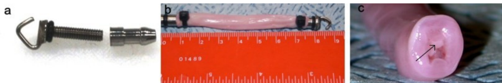
Figure 4.3: (a) Novel design of an adapter to facilitate handling and seeding of HUV. (b) HUV seeded with collagen and MSCs and cultured for 1 week. (c) Cross section of seeded HUV 1 week post-culture. Arrow points to cellular collagen hydrogel that was injected in the center of the HUV.
