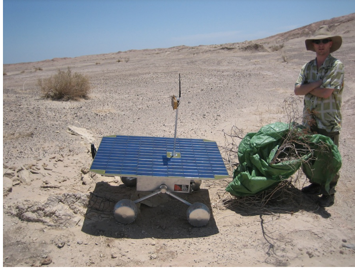
Figure 2.5: The green tarp is used to create more surface area over vegetation for the range finders to obtain proper readings.
