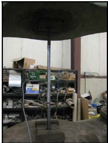
Figure 4.4: Tensile strength testing of longitudinal deformed bar
