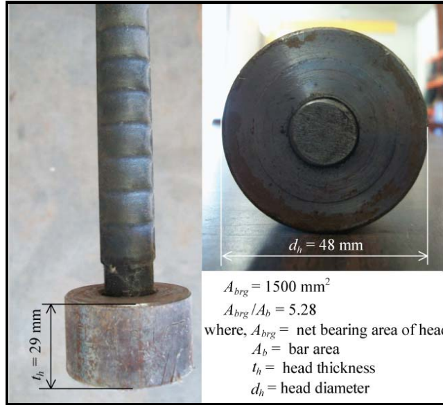
Figure 6.2: Heads and threaded connections (Conversion: 1 mm = 0.039 in.)
