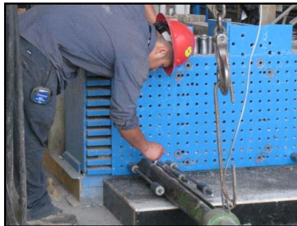
(a) Prestressing of 13 mm ( \frac{1}{2} in.) diameter low relaxation strands with a hydraulic jack
