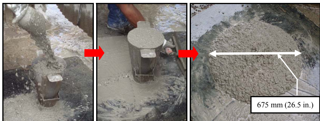
Figure 5.3: Slump flow test
