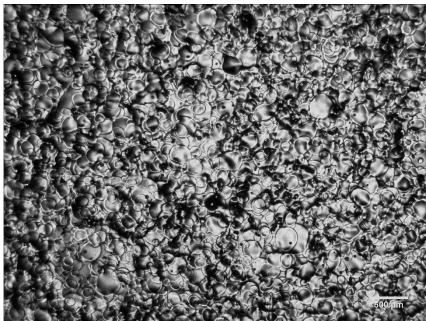
Figure 32 40X image of the 2% film (29% energy, 80°C, 150μL/min)
