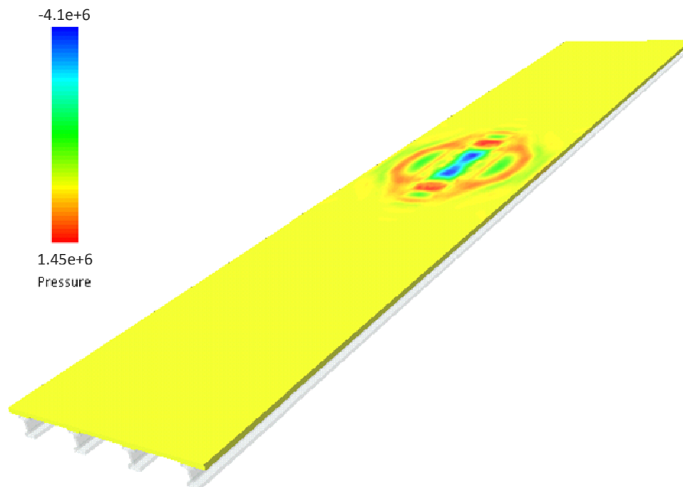
Figure 6.29: Superstructure Pressure (Pa) 6 ms After Blast Initiation
