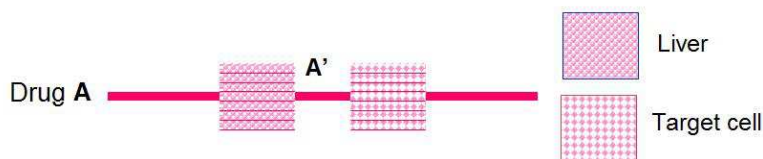
Figure 1. Perfusion system for metabolism-dependent toxicity study (A' is the converted drug by liver metabolism).
