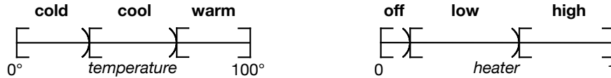
Figure 3.1: The crisp variables temperature and heater are used by a controller for a heater. The temperature crisp variable is an input value to the controller and has three values: cold , cool , and warm . The heater crisp variable is an output value from the controller and denotes the desired power level of the heater. It has three values: off , low , and high .
