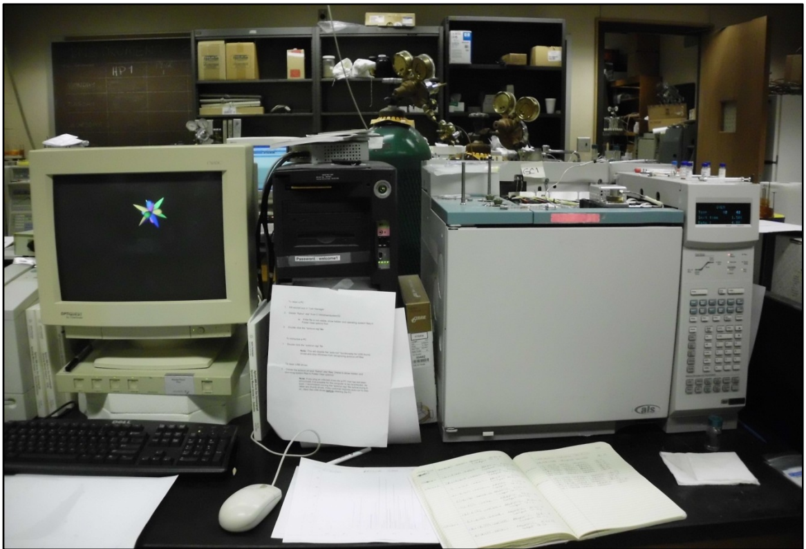
Figure 3.6. Gas chromatography (GC-FID) (Hewlett-Packard 35141) used in the study. Organic Geochemistry Laboratories, University of Oklahoma.
