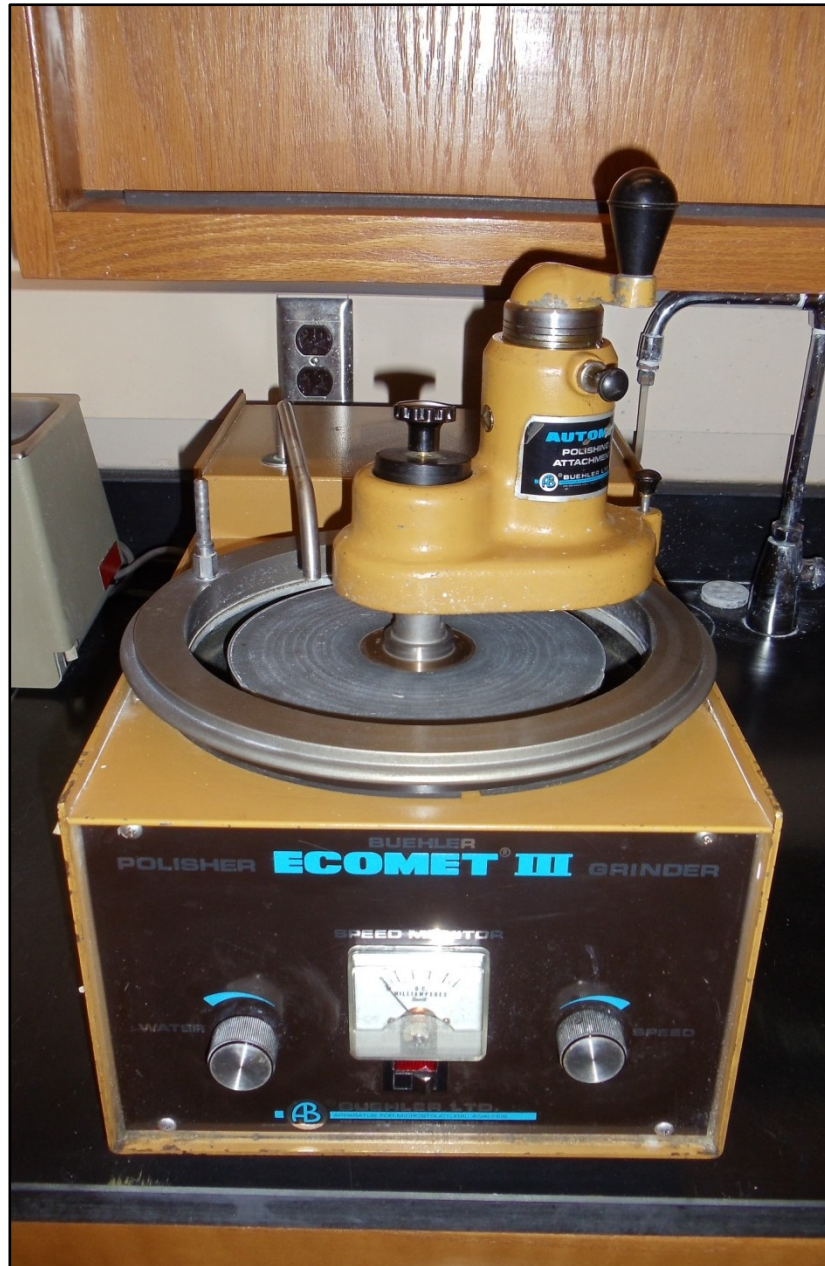
Figure 3.4. Buehler Ecomet III Grinding and Polishing Apparatus used for polishing dispersed organic pellets. Organic Petrology Laboratory, Oklahoma Geological Survey, University of Oklahoma.
