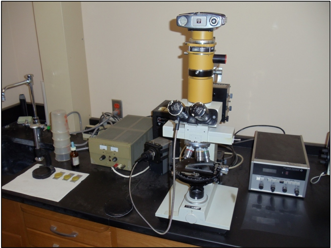
Figure 3.5. A Vickers M17-Photomicroscope used for graptolite reflectance study. Organic Petrology Laboratory, Oklahoma Geological Survey, University of Oklahoma.
