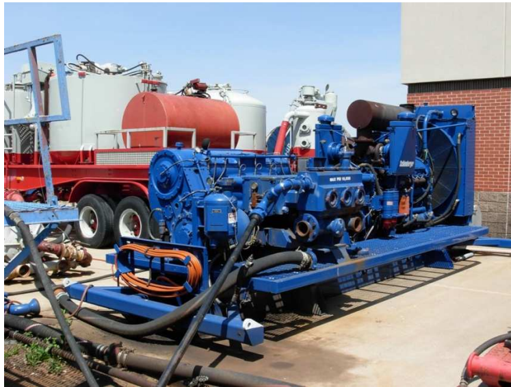
Figure 4.4 Schlumberger B804 triplex plunger pump.
