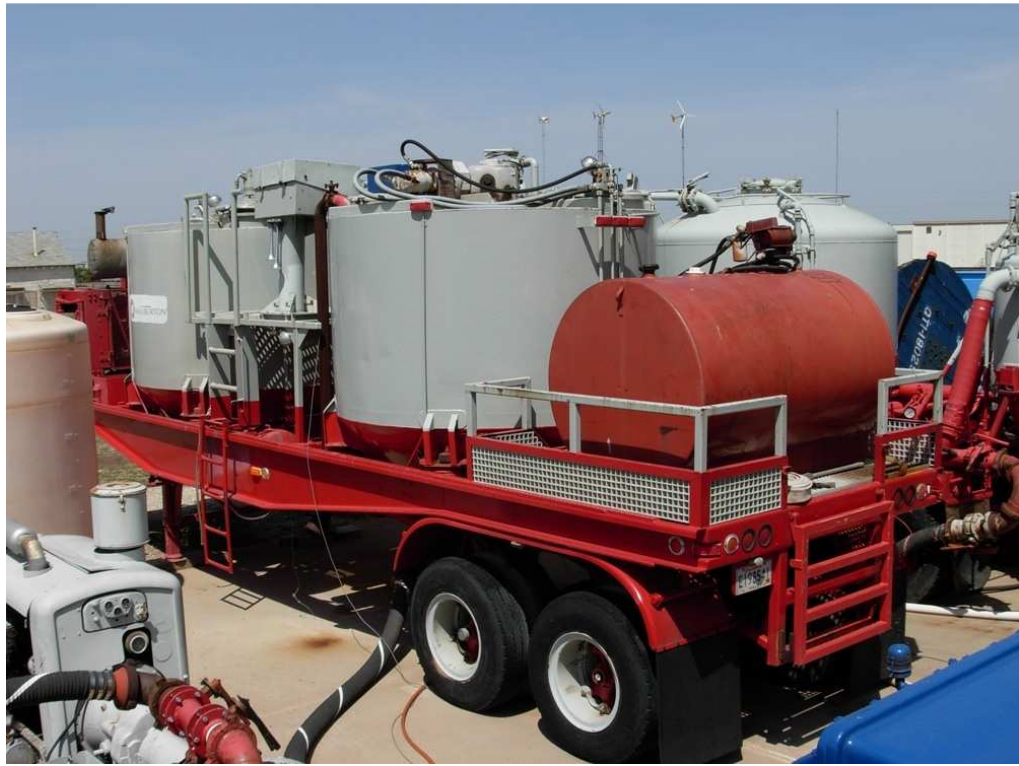
Figure 4.3 Two 50-bbl fluid mixing and storage tanks.
