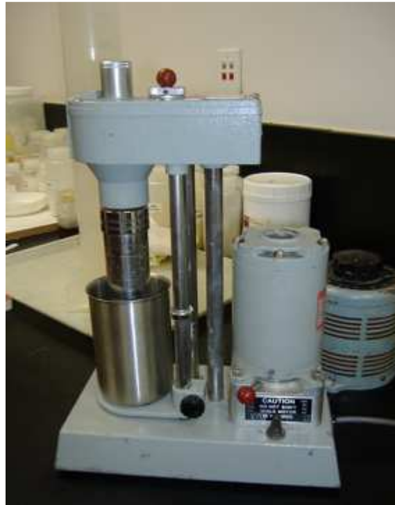
Figure 4.6 Fann Model 35 Viscometer.
