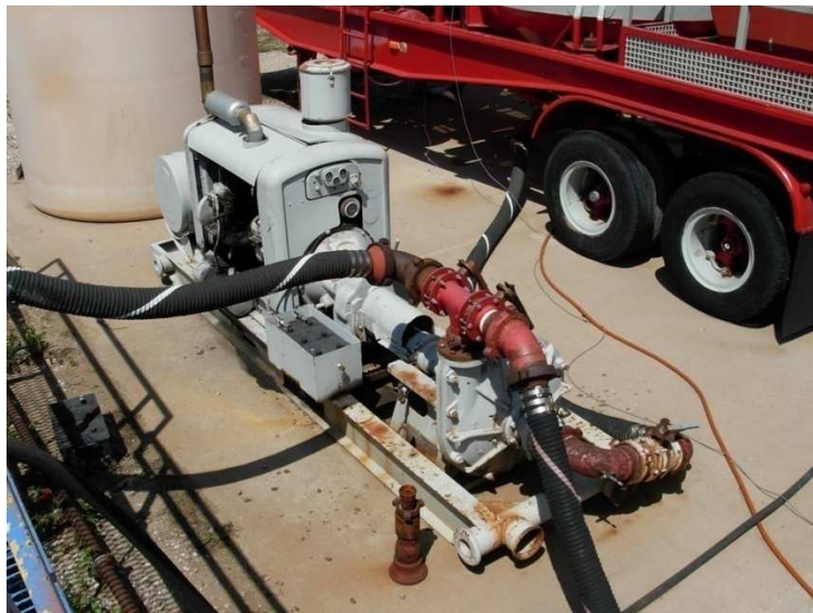
Figure 4.5 Galigher centrifugal pump.
