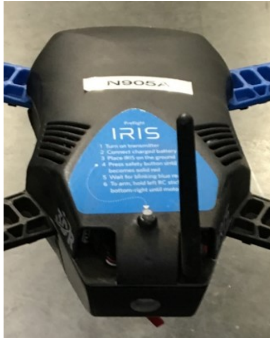
Figure 2.2: Antenna configuration of the included coiled monopole rubber duck antenna on the IRIS craft used as an antenna test platform [17]
