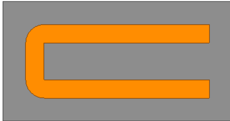
Figure 4.9: Planar U-shaped patch
