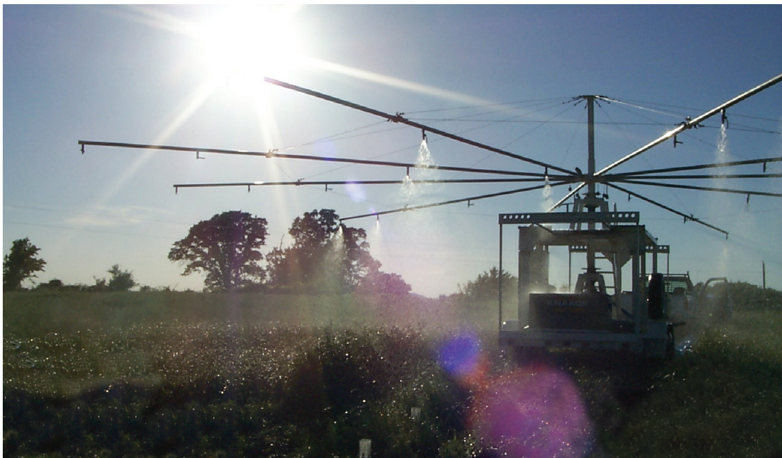
OSU Researchers use rainfall simulator to investigate phosphorus BMPs for pasture systems.
