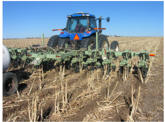
Figure 6. Applying anhydrous ammonia with strip-till implement in the early spring.
