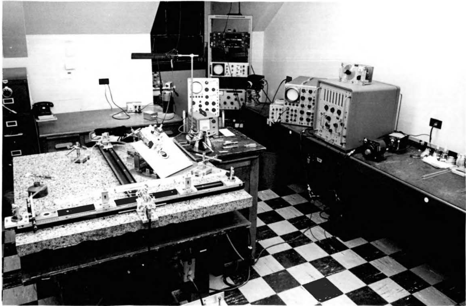
Figure 9. Equipment in the Configuration Used While Taking Beat Frequency Measurements
