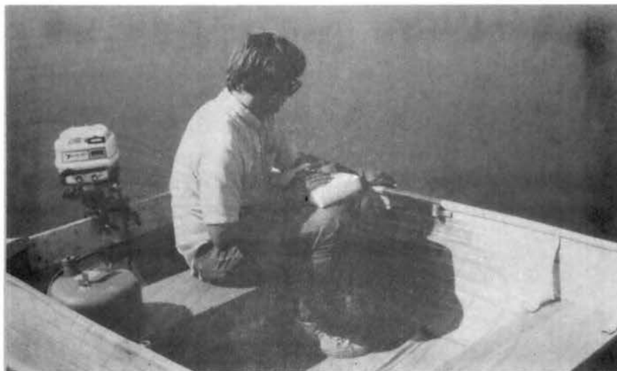
Figure 21. Measuring DO and Temperature Profiles with Electronic Monitor
