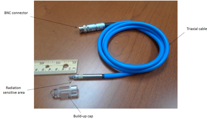
Figure 7.1: PTW TN31014 ionization chamber.
